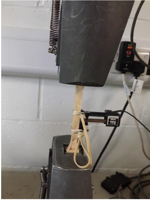
Figure 6.32 Picture of the tensile test arrangement
