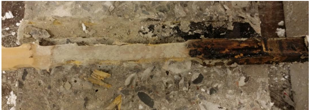
Figure 5.5 Picture of the bamboo-concrete surface after failure for linseed treated splint (Tr 2 mm 1:1.5)
