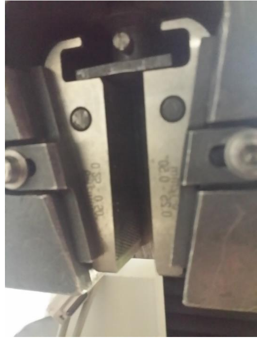
Figure 6.33 Picture of the tensile test's machine grip
