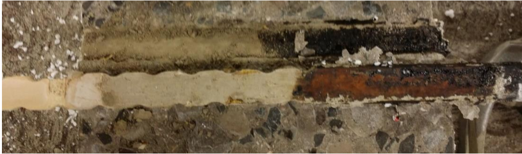
Figure 5.7 Picture of the bamboo-concrete surface after failure for an untreated splint (2 mm 1:1)
