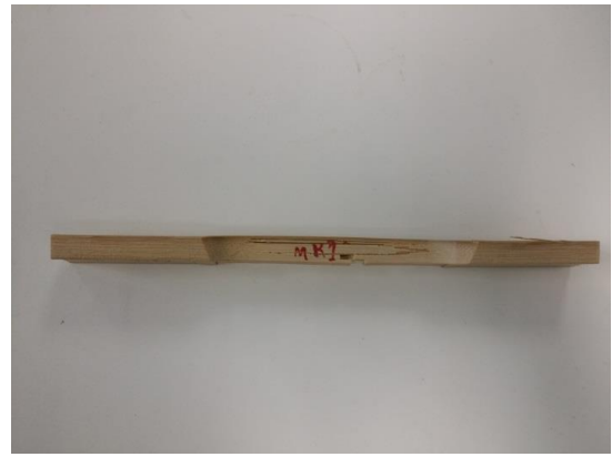
Figure 6.39 Picture of typical failure of Moso 1:3 ratio (side view)
