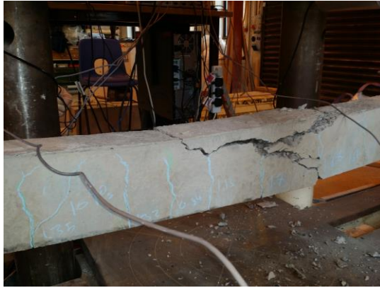
Figure 6.10 Picture showing compression failure of Beam 8
