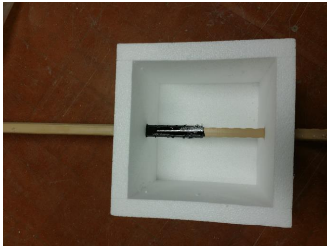
Figure 5.1: Picture of a splint in the form with bitumen-based debonding compound
