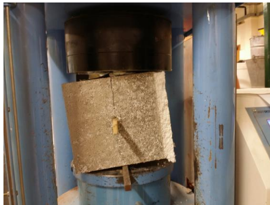
Figure 5.4 Picture of the splitting of pull-out specimens
