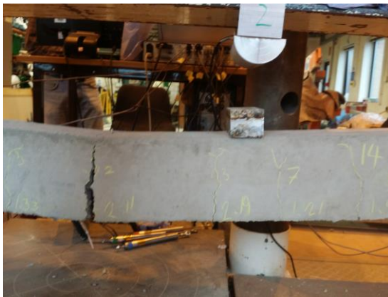
Figure 6.12 Picture showing the bond failure of Beam 14
