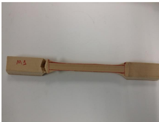
Figure 6.34 Picture of typical failure of Moso 1:2 ratio (top view)
