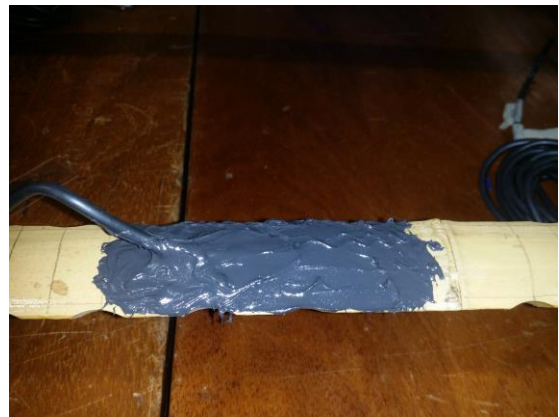
Figure 6.13 Picture of the strain Gauge protection material
