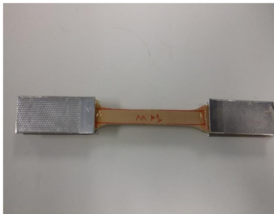
Figure 6.36 Picture of typical failure of Moso 1:2 ratio + Aluminium tabs and epoxy (top view)
