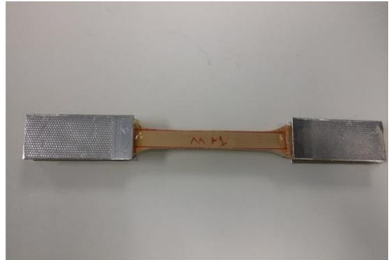
Figure 6.31 Picture of the use of tabs and epoxy for bamboo tensile test specimens
