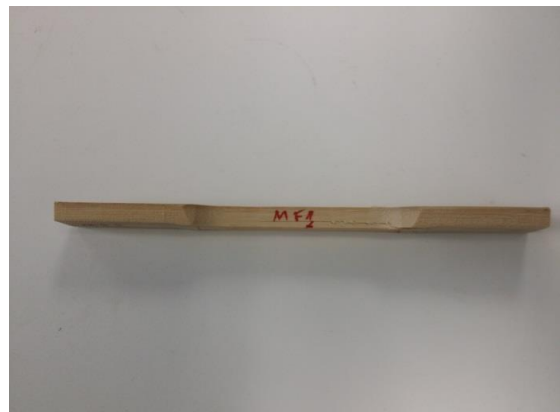
Figure 6.41 Picture of typical failure of Moso with flattened ends, 1:2 ratio (side view)
