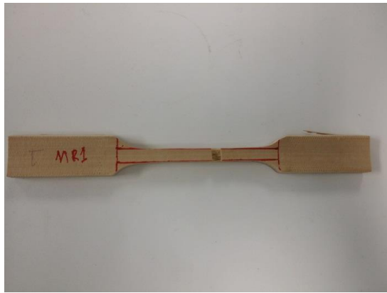
Figure 6.38 Picture of typical failure of Moso 1:3 ratio (top view)
