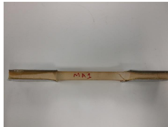
Figure 6.37 Picture of typical failure of Moso 1:2 ratio + Aluminium tabs and epoxy (side view)
