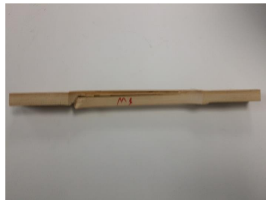
Figure 6.35 Picture of typical failure of Moso 1:2 ratio (side view)
