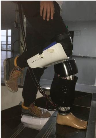
Fig. 13. Human-walking experiment under stairs
