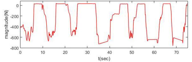
Fig. 15. Ground reactive force under stair ascent and descent
