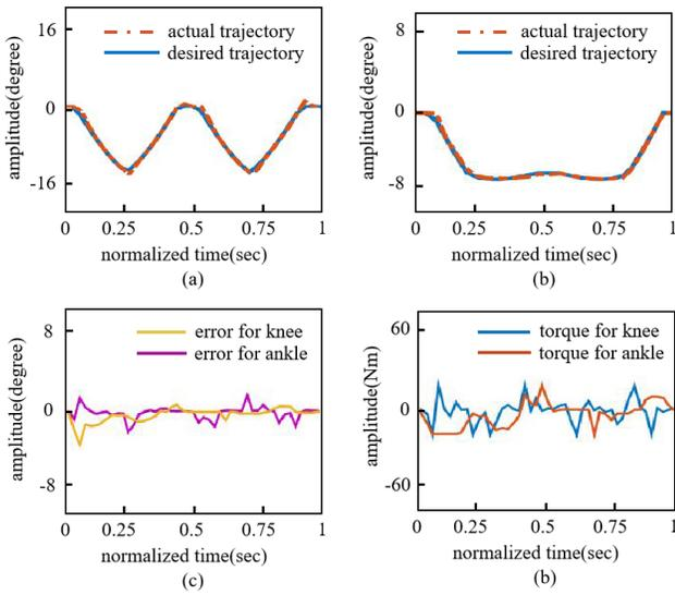
Fig. 11. Experimental results of subject 3.(a)The tracking trajectory of knee joint.(b)The tracking trajectory of ankle joint.(c)The trajectory error.(d)The torque of each joint
