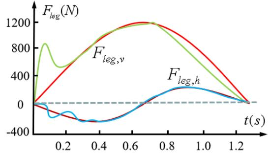
Fig. 1. Ground reactive force (GRF) of the contralateral leg during stance phase
