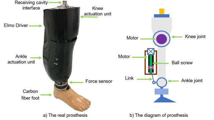
Fig. 6. The mechanical structure of the leg prosthesis
