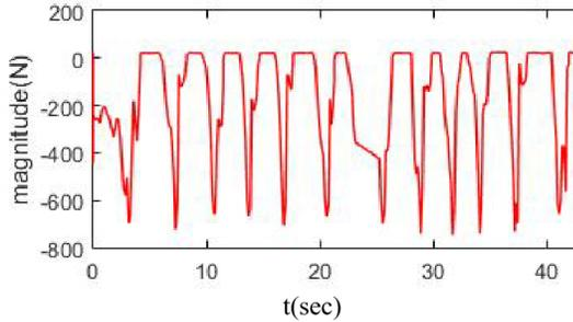
Fig. 12. Ground reactive force under level ground
