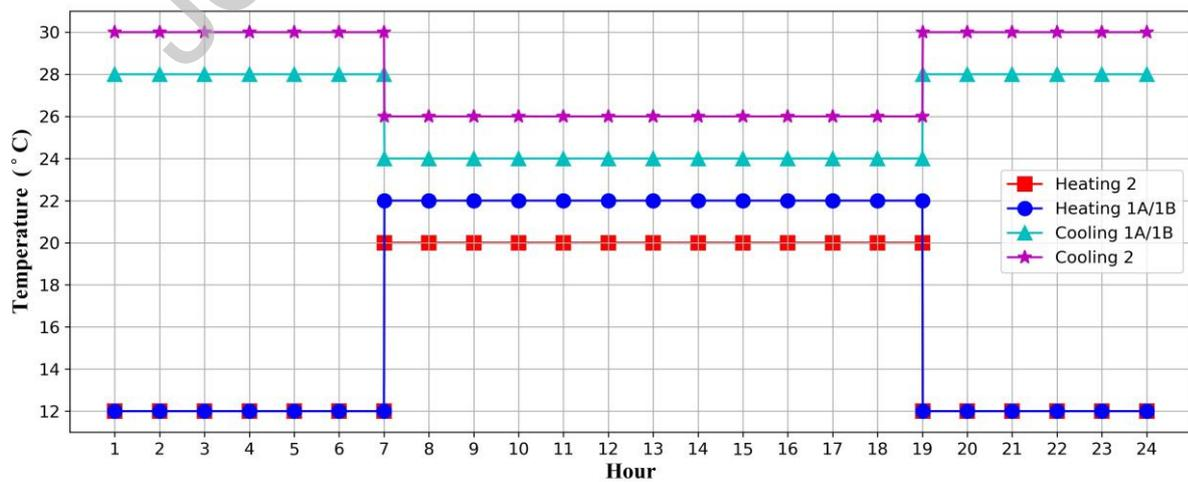
Fig. 6. Temperature setpoints of heating and cooling on the weekdays.
