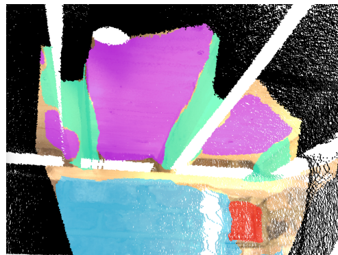
Figure 16: Example of mapping the 2D labels onto a region of a 3D point cloud (here LiDAR data).
