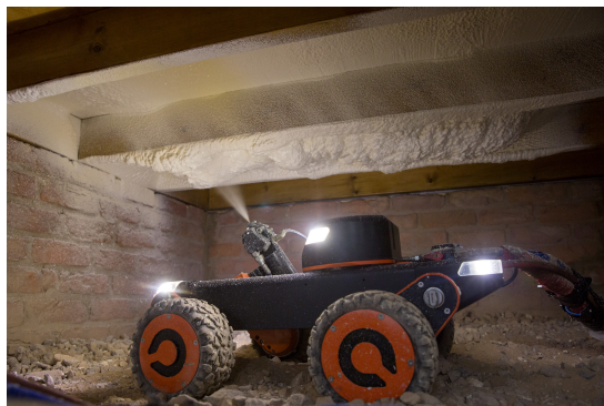
Figure 1: Photograph of the robot used for data capture, shown here applying insulation foam to illustrate an application. The robot dimensions are approximately 58cm(L), 45cm(W), 29cm(H).
