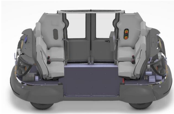
Figure 6. Cutaway of shuttle seating arrangement. Photo credit: Westfield Technology Group.
