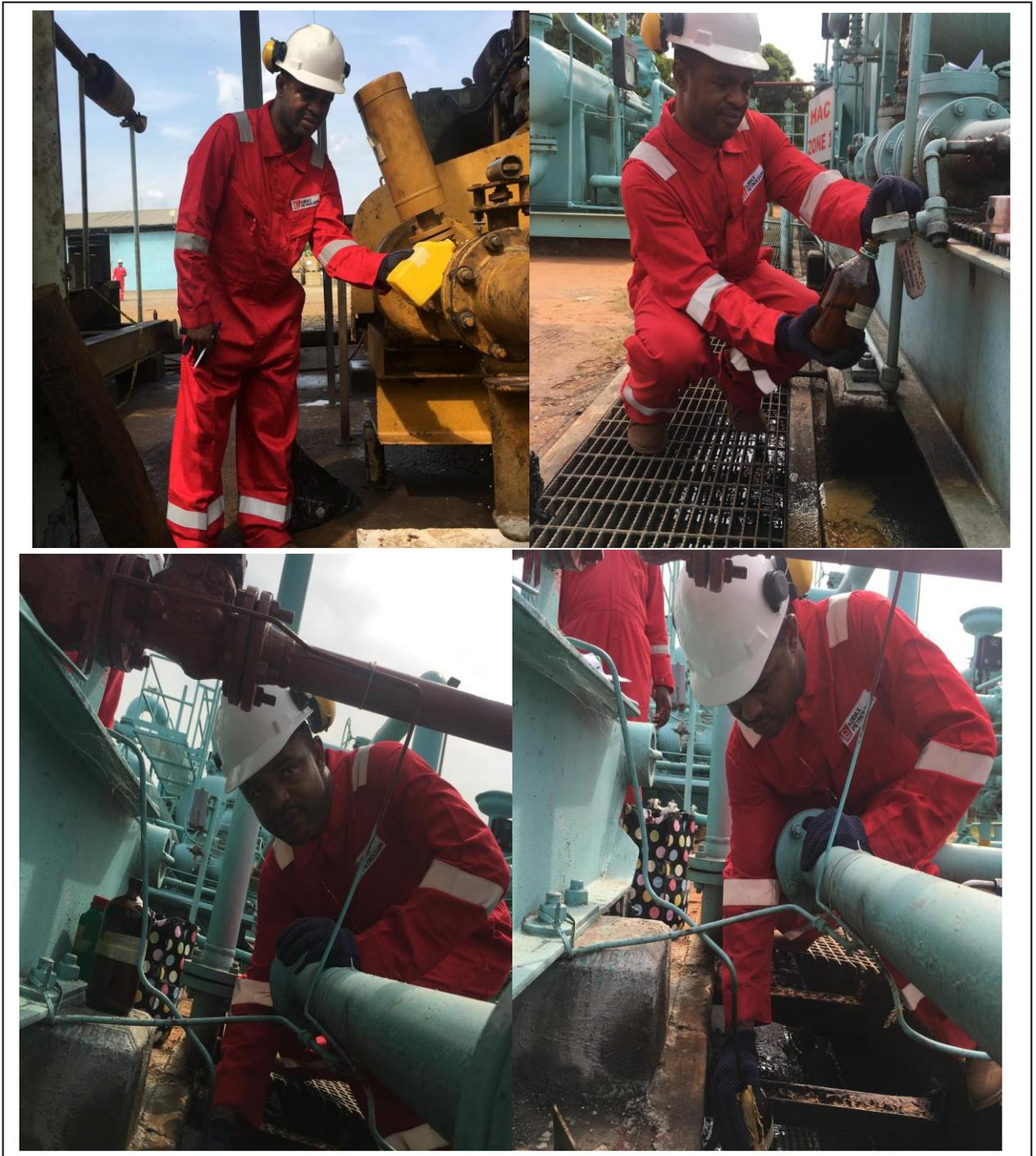
Pic E 2: Sample Collection at Different Sampling Points in Crude Oil Production Facilities in Nigeria
