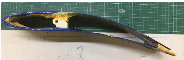
Figure 5. Final manufactured prototype at max camber
