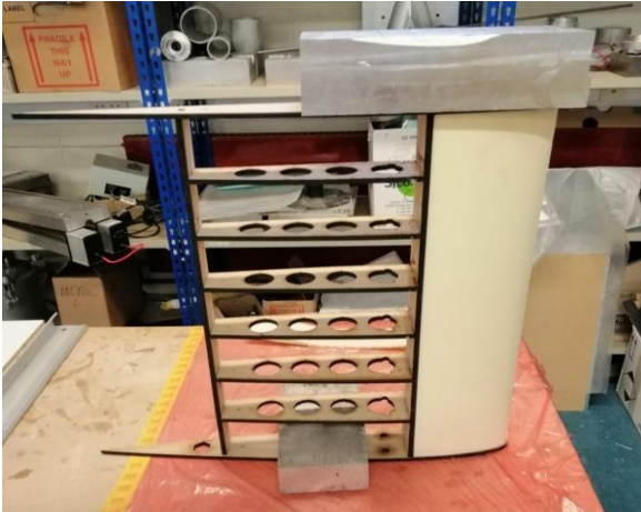
Figure 9. Internal and assembly of final prototype
