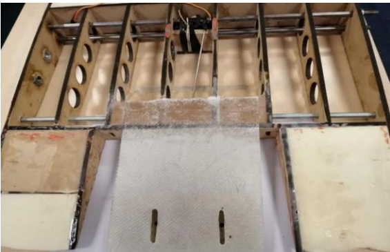
Figure 11. Adjusted internal morphing flap wing
