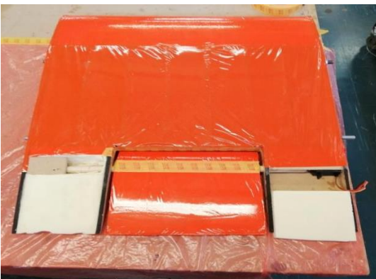
Figure 10. Single hinged flap wing
