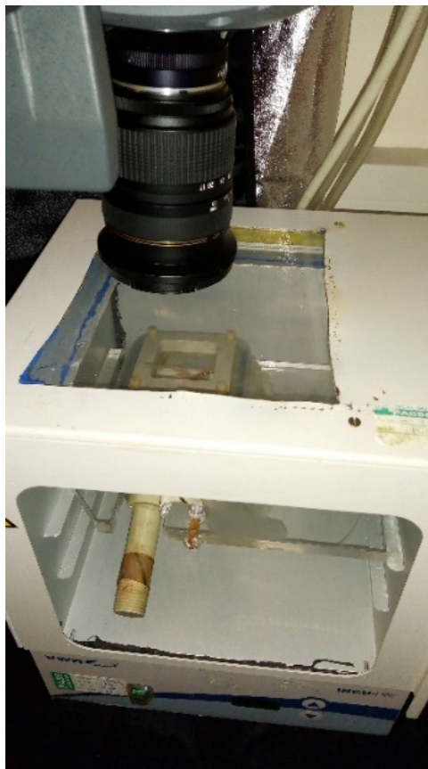
Figure 3.5: Modifications to allow the use of bioluminescence reporter organisms in the flat plate biofilm model
