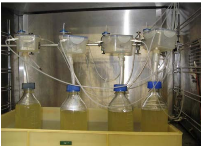
Figure 3.1: Several biofilms incubated in a single large incubator with fan circulation
