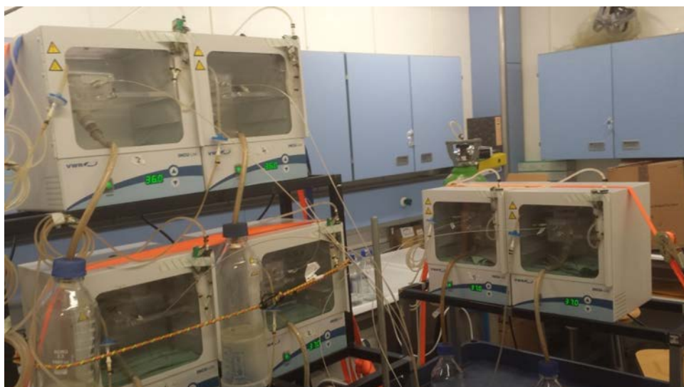
Figure 3.8: Six incubators showing equal length PEEK tubing entering each through the front panel.
