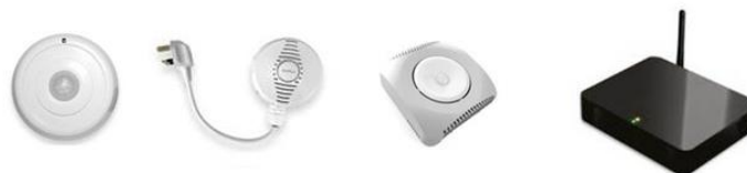
Figure 26 HeatingSave sensors and hub
