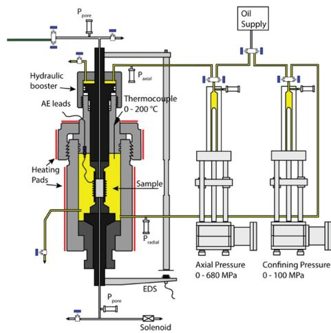
Figure 1 Triaxial cell used in this work, adapted from Fazio *et al.* 2019
