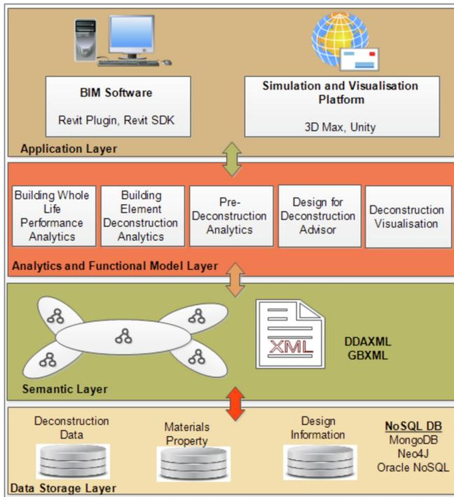
Fig. 2. Disassembly and deconstruction analytics system (D-DAS) architecture.
