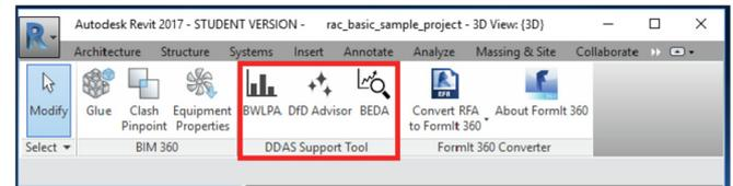
Fig. 4. D-DAS implementation plug-in in Autodesk Revit 2017
