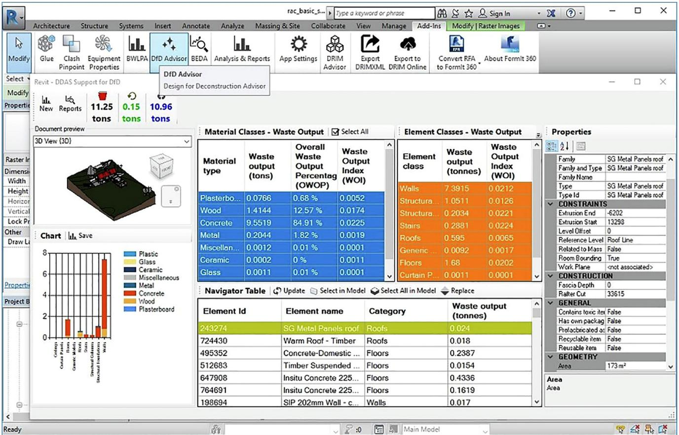
Fig. 7. Design for deconstruction advisor implementation in Autodesk Revit 2017.
