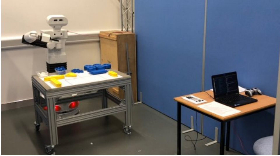
Figure 1: Experimental setup for Study 1. Participants are sat in front of the robot; the wizard is sitting behind the participants, out of their field of view. The robot guides the assembly of a toy car by the participant, using the parts displayed on the table.
