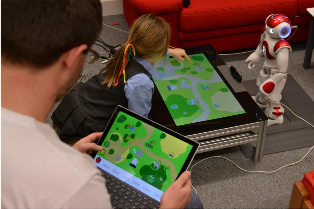
Figure 2: **Setup used in the study.** A child interacts with the robot tutor, with a large touch-screen sitting between them, displaying the learning activity; a human teacher provides guidance to the robot through a tablet and monitors the robot’s learning. While the picture depicts an early lab pilot, the main study was conducted on actual school premises.
