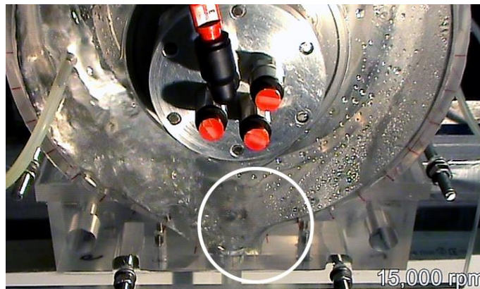
FIGURE 9: UPSTREAM FLOW DETACHMENT WAS NOT OBSERVED.
