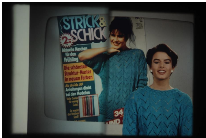
Figure 1. “Butterfly screening” of a chromogenic print: analog projection on the left (Kinoton FP38) and digital projection on the right (Christie CP2210). The sliding cut is achieved with a curtain mounted on a rail.
