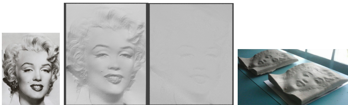
Figure 1: example of gray-levels pattern to be displayed, realistic simulation with oriented illumination, same simulation with isotropic lightning, physical realization in concrete for the 2017 Lima Design Week, Perú.
