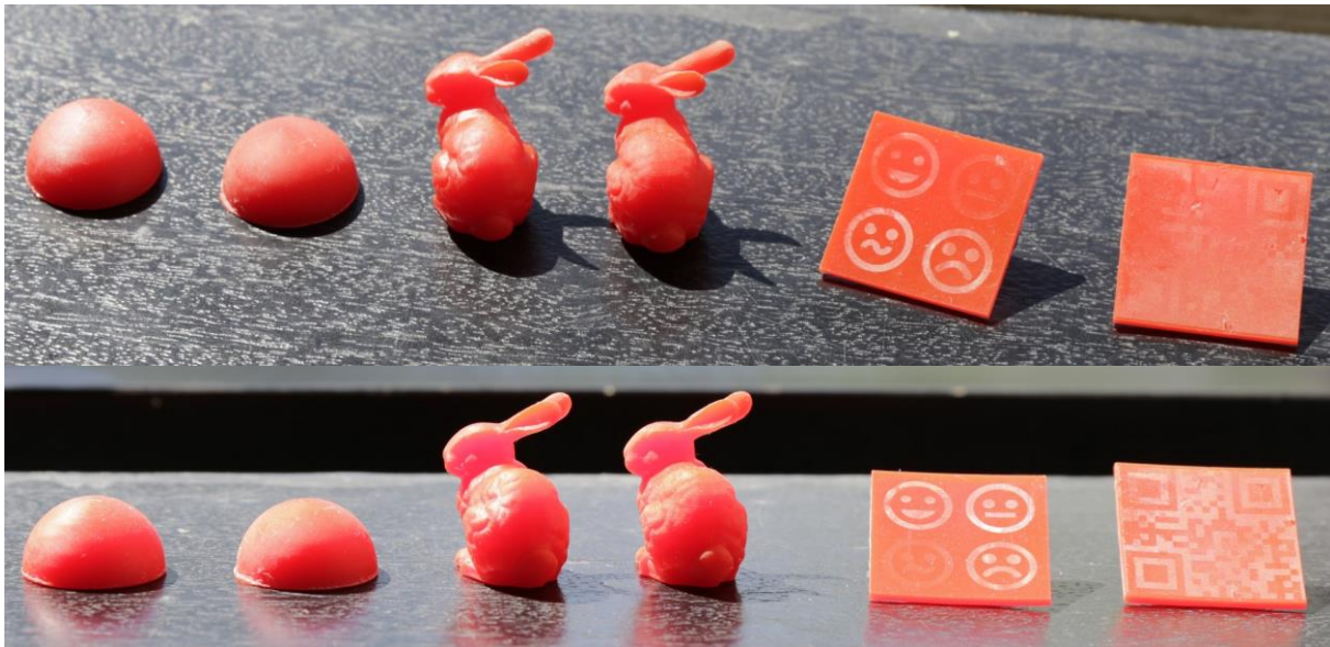
Figure 1. Hemispheres and bunnies with smooth and rough surfaces. Flat samples (smileys and QR code) with spatially varying anisotropic reflectance. The scene is observed from two directions to exhibit the anisotropy. The sun is the light source. Each item was printed in a one-step process using the presented technique.
