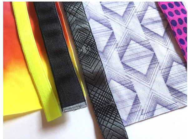
Fig. 1. Laser peri-dyed design and coloration effects on: intimate apparel polyester fabrics; nylon-elastane knitted sportswear fabrics; and narrow band nylon-elastane straps.
