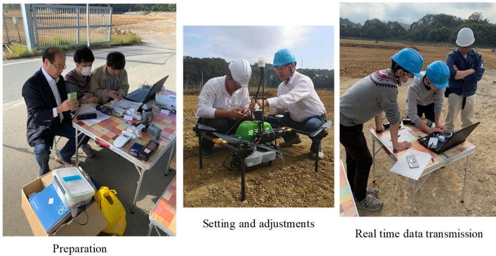
Figure 4: Observation using UAVs with the sensors of PM_{2.5} , PM_{10} , and O_3 at Yorrii-machi rural site, Saitama prefecture, Japan on November 15, 2018.
