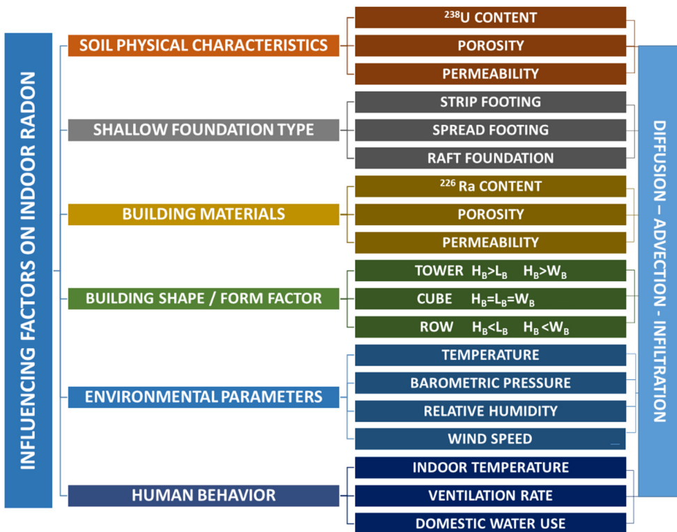
Figure 1: Summary of the interaction among the numerous parameters that affect indoor radon concentration levels.
