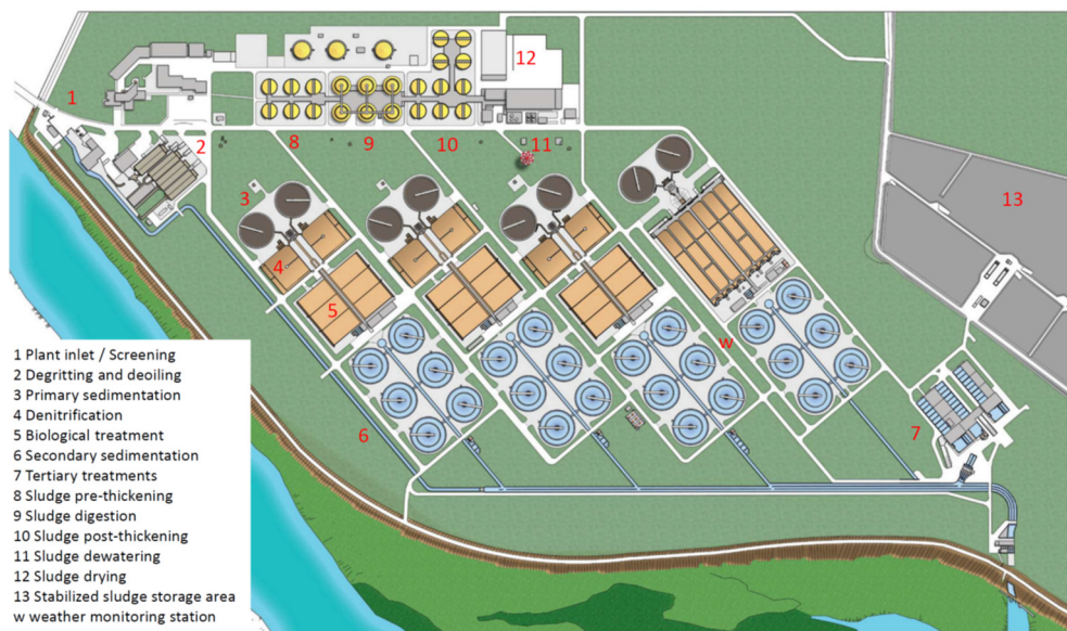
Figure 1: Plant of SMAT's WWTP [9].
