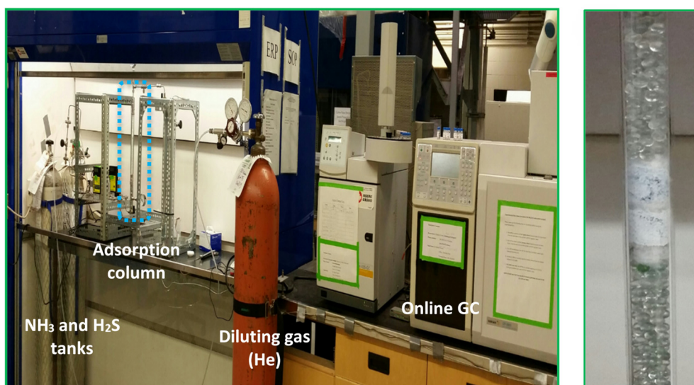
Figure 2: Experimental set-up (left). Adsorption column packed with \text{ZnO} and \text{TiO}_2 nanoparticles and glass beads (right).
