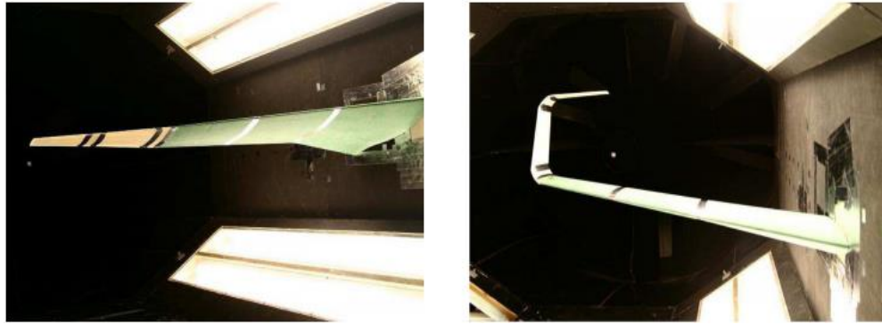
Figure 2.29: Aircraft wing with a morphing wing tip (Gabor et al. 2016). (Used with permission of the publisher)
