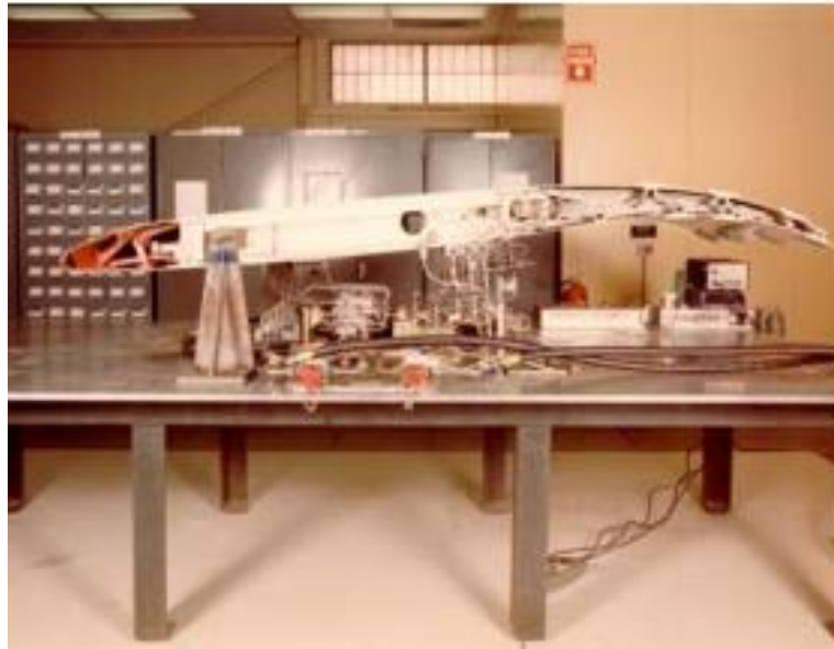
Figure 2.9: MAW airfoil cross-section in its deformed, cambered position (Weisshaar, 2006).©NASA
