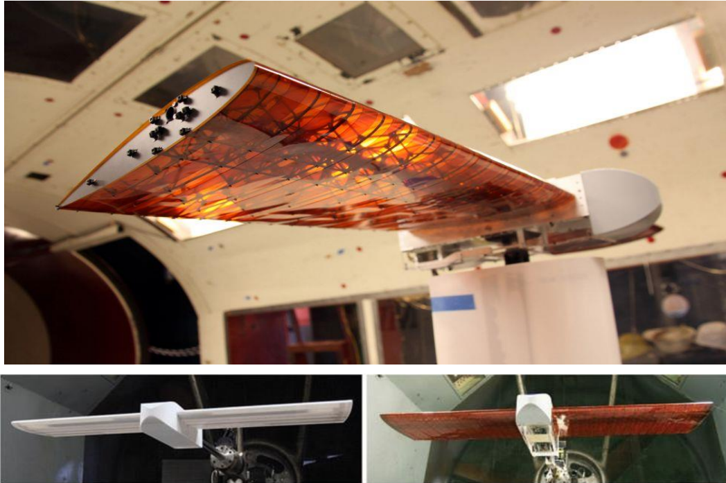
Figure 2.14: Testing setup in NASA Langley wind tunnel. (Lower Left) Rigid wing model. (Lower Right) Flexible wing model (Jenett et al., 2016). (Used with permission of the publisher)
