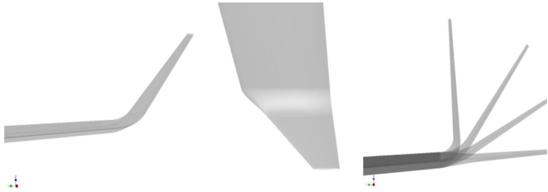
Figure 2.22: Morphing wingtip design investigated using DLM (Cooper et al. , 2015). (Used with permission of the publisher)
