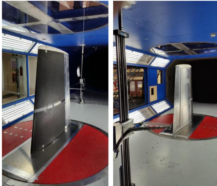
Figure 2.25: MDO505 wing model setup in a wind tunnel test section (Gabor et al., 2016). (Used with permission of the publisher)
