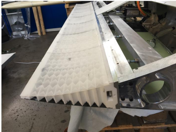
(a) The integrated actuation mechanism in the blade section.
