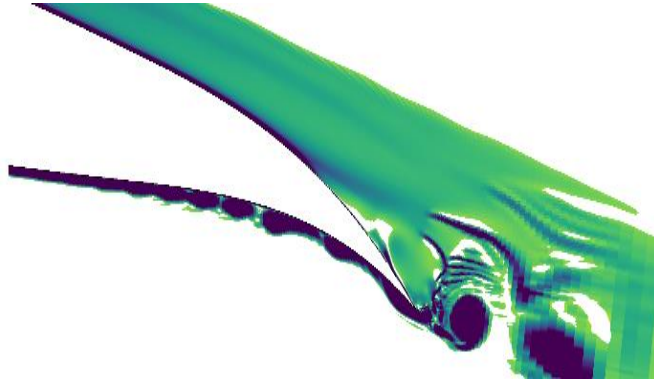
Figure 5.7: Close-up showing the flow features around the TE and the formation of LBL at the pressure surface.
