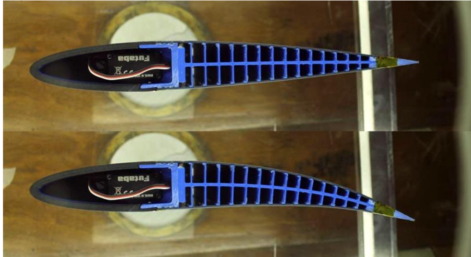
Figure 2.27: FishBAC wind tunnel model: (top) baseline state (lower) deformed state (Woods et al., 2013). (Used with permission of the publisher)
