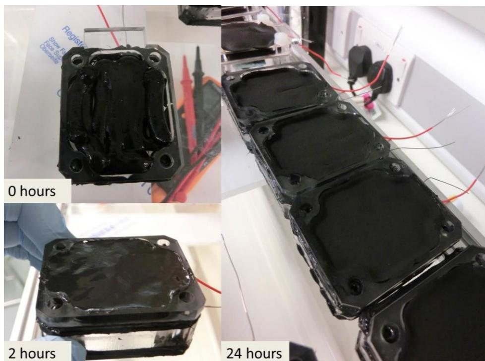
Figure 4.22 - Manually extruded PTFE-free alginate electrode 0, 2 and 24 hours after extrusion, showing the electrode settling and solidifying (air-drying).
