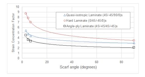
Figure 9: Plot of strain concentration against scarf angle for three types of laminates,
