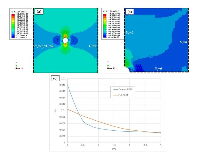
Figure 2: Strain ( $\varepsilon_{xx}$ ) contour plot and boundary conditions of; (a) full scarf FEM; (b) a quarter scarf FEM; (c) strain ( $\varepsilon_{xx}$ ) plots along the line of symmetry for both models for stacking sequence [45/-45/90/0]<sub>s</sub>
