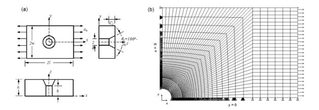
Figure 1: Configuration of (a) countersunk hole and (b) a quarter FEM (28)
