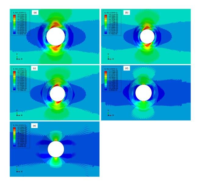
Figure 11: Strain in loading direction for scarf angle of 7° and stacking sequences (a)  $[45/-45/90/0]_s$ , (b)  $[45/-45/0/90]_s$ , (c)  $[45/0/-45/90]_s$ , (d)  $[0/45/-45/90]_s$  and (e)  $[0_4]_s$  (loading is in direction of x axis)
