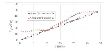
Figure 4: Distribution of homogenised modulus of elasticity in load bearing direction,  $E_x$ , in the scarf region for scarf angle of 3° and stacking sequence [45/-45/90/0]<sub>s</sub>
