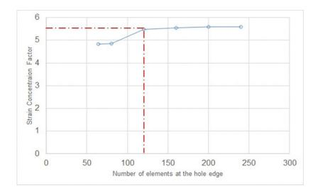
Figure 7: Graph of mesh sensitivity study for scarf angle of 3° and stacking sequence
