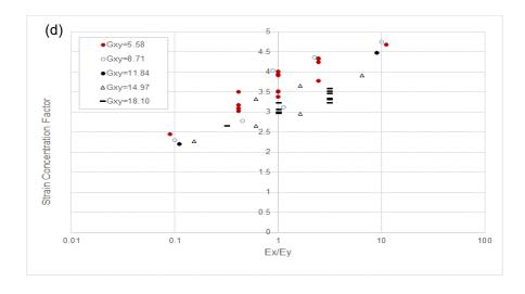
Figure 8: Semi-logarithmic plots of STRCF versus ratio of homogenised modulus of elasticity for various homogenised shear modulus and scarf angles (a) 3°, (b) 5°, (c) 7° and (d)
