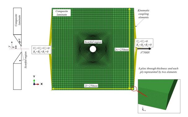
Figure 5: Representation of the scarfed composite structure (scarf angle of 3°) for FEA
