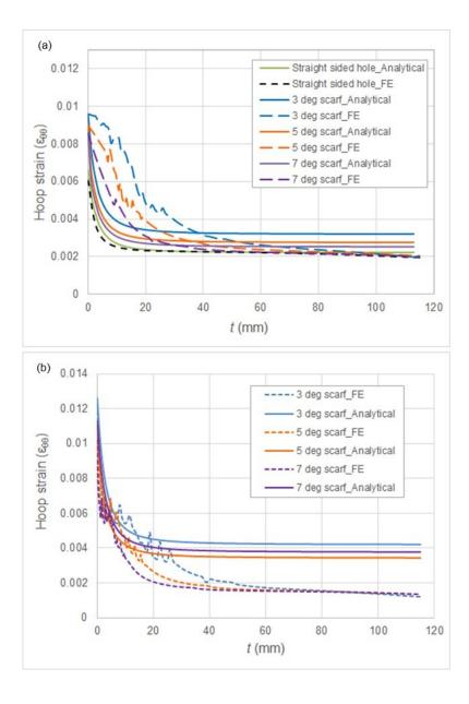
Figure 3: Hoop strain distribution vs the distance from the edge of the hole for scarf angle of 3°, 5°, 7° and straight sided hole with stacking sequences; (a) quasi-isotropic laminate of [45/-45/90/0]<sub>s</sub>, (b) hard laminate of [0/45/-45/0]<sub>s</sub>
