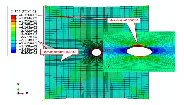
Figure 6: Contour plots of strains in x direction ( $\varepsilon_{xx}$ ) for straight sided hole and stacking sequence of [45/-45/0/90]<sub>s</sub>
