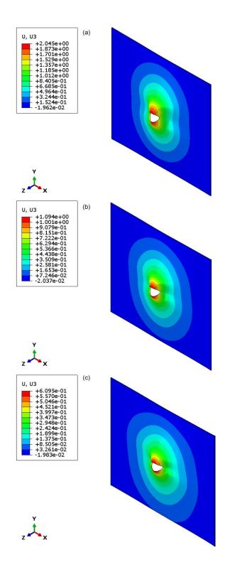
Figure 10: Out of plane deformation of scarfed laminates for scarf angles (a)  $3^\circ$ , (b)  $5^\circ$  and (c)  $7^\circ$  (loading is in direction of x axis and all dimensions are in millimetres)
