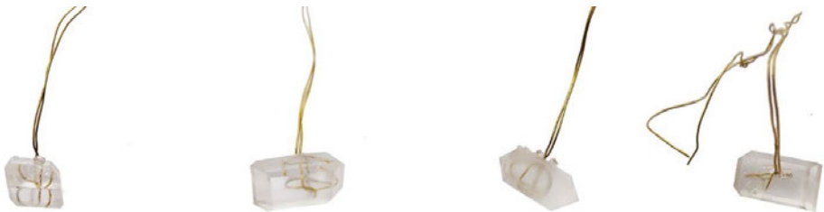
Figure 3: Various Views of a Grown Single Sugar Crystal with Brass Wire Inclusion Source: Boons
