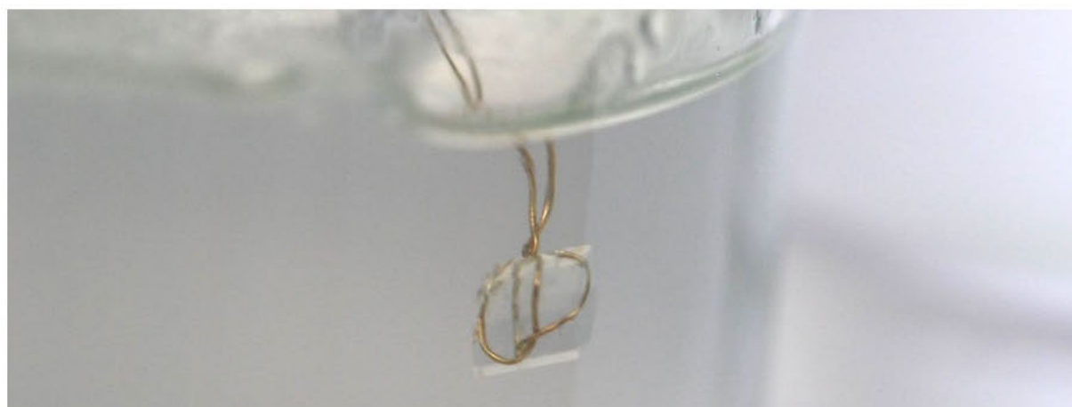
FIGURE 11. Single sugar crystal suspended from brass wire in supersaturated sugar solution.
