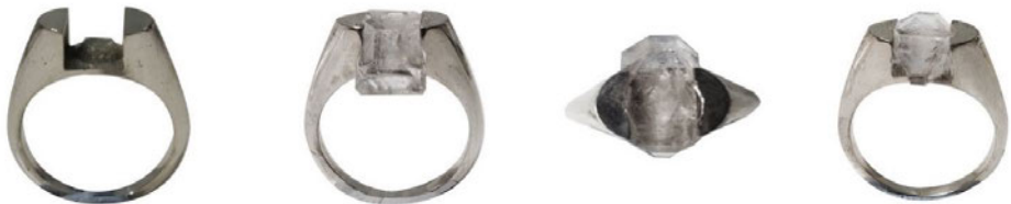
Figure 4: Silver Ring with In Situ Grown Alum Crystal from Various Views: Before-Growth Images on the Left and After-Growth Images on the Right Source: Boons
