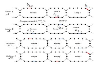
Fig. 4. Crossover with one point in three independent loops (---- open arc in Parent 1 chromosome, ---- open arc in Parent 2 chromosome)
