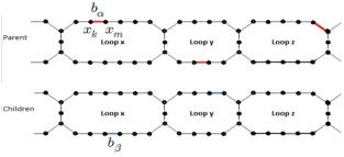
Fig. 3. Mutation in three independent loops (---- open arc in children chromosome, ---- open arc in parent chromosome)
