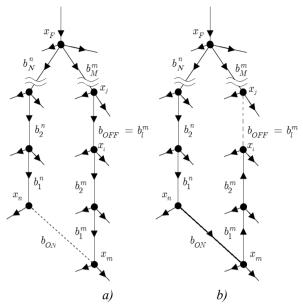
Fig. 2. Branches exchanging  $s^{\text{(new)}} = s^{\text{(old)}} \otimes (b_{\text{ON}}, b_{\text{OFF}})$ a) configuration  $s^{\text{(old)}}$  b) configuration  $s^{\text{(new)}}$
