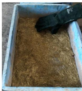
**Figure 2.** Steel fiber used in this study.
