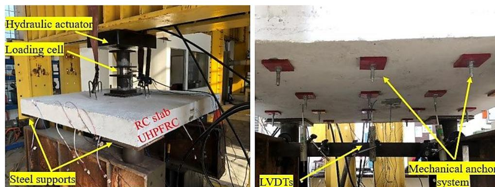
Figure 6. Test setup and instruments applied to specimens.
