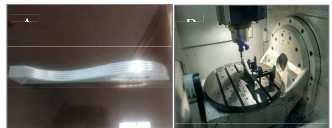
Fig. 12. The experiments performed on the 5-axis CNC machine “Spinner U5-620”. (A): The machined part. (B) The machined part which is fixed on the machine table.
