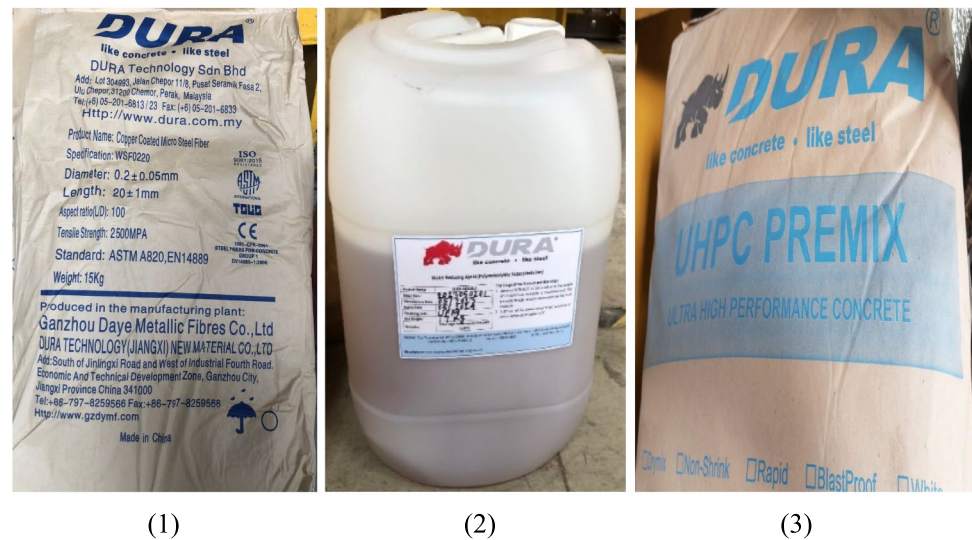
Fig. 2 Main ingredients of the UHPFRC; (1) steel fiber, (2) admixture for reduction of water, and (3) UHPC premix Dura
