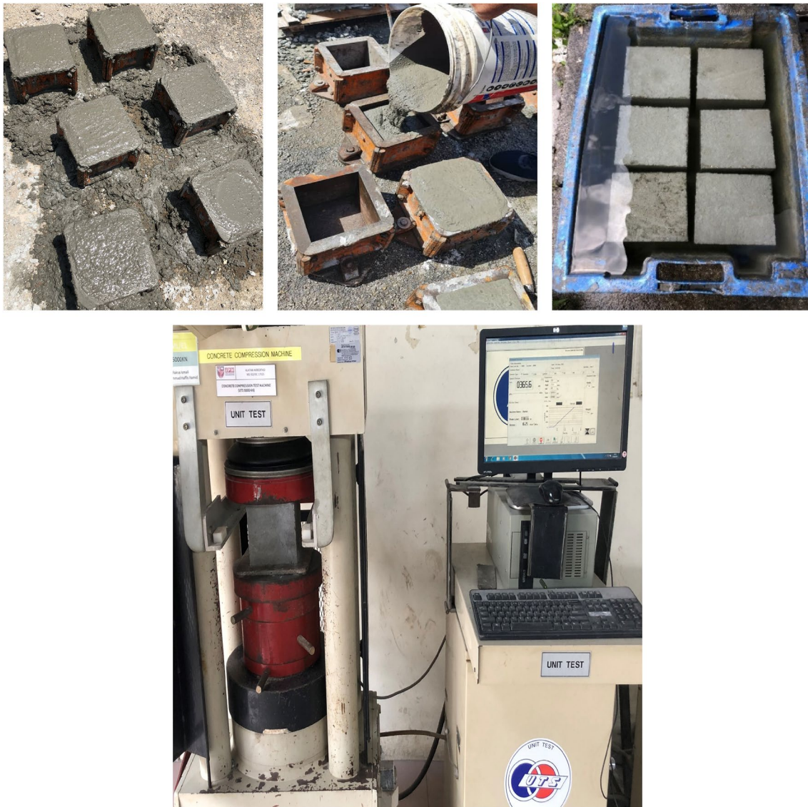
Fig. 4 NC and UHPFRC property evaluation and test
