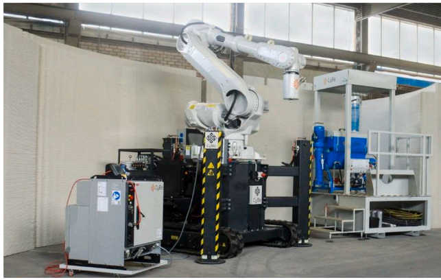
Fig. 8. Robotic arm 3D-printing system.
