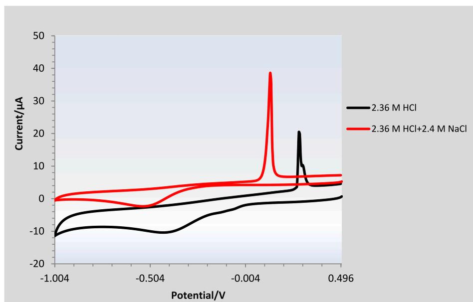
Fig. 6. Cyclic voltammetric behaviour of 20 mg/l  $\text{Hg}^{2+}$  in 2.36 M HCl in the presence of 2.4 M NaCl and the absence of NaCl. Starting potential, +0.5 V; scan rate  $50 \text{ mVs}^{-1}$  switching potential,  $-1.0 \text{ V}$ .
