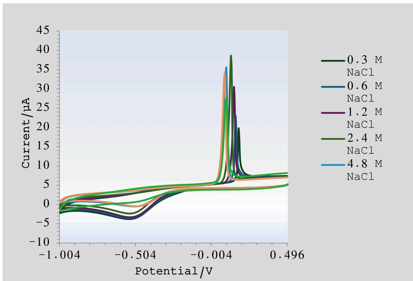
Fig. 4. Cyclic voltammetric behaviour of 20 mg/l  $Hg^{2+}$  in 2.36 M HCl in the presence of varying concentrations of NaCl. Starting potential, +0.5 V; scan rate 50  $mVs^{-1}$  switching potential, -1.0 V. The highest stripping peak was observed in 2.4 M NaCl.
