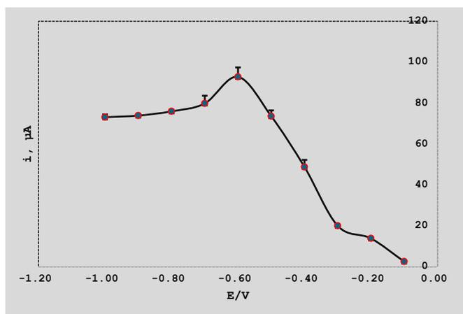
Fig. 7. Effect of deposition potential on the DPASV of  $\text{Hg}^{2+}$  at 20 mg/l in 2.36 M HCl and 2.4 M NaCl. Deposition time, 60 s, and scan rate  $50 \text{ mVs}^{-1}$ . Error bars represent SEM.
