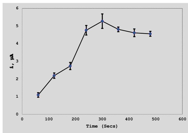
Fig. 8. Effect of deposition time on the DPASV of  $\text{Hg}^{2+}$  at 20 mg/l in 2.36 M HCl and 2.4 M NaCl. Deposition potential  $-0.6 \text{ V}$ , and scan rate  $50 \text{ mVs}^{-1}$ . Error bars represent SEM.
