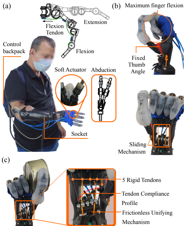
Fig. 1. PrHand V3 underactuated Soft-Robotic prosthetic hand. a) Amputee user adaptation and illustration of finger flexion and extension (a tendon-driven compliant mechanism) and abduction degree of freedom driven by a soft silicone actuator. b) PrHand V3 prosthesis enhancements. c) Compliant grip example showing how a compliant profile is generated in the elastic tendons, adapting to the shape of the object gripped without needing prior control.
