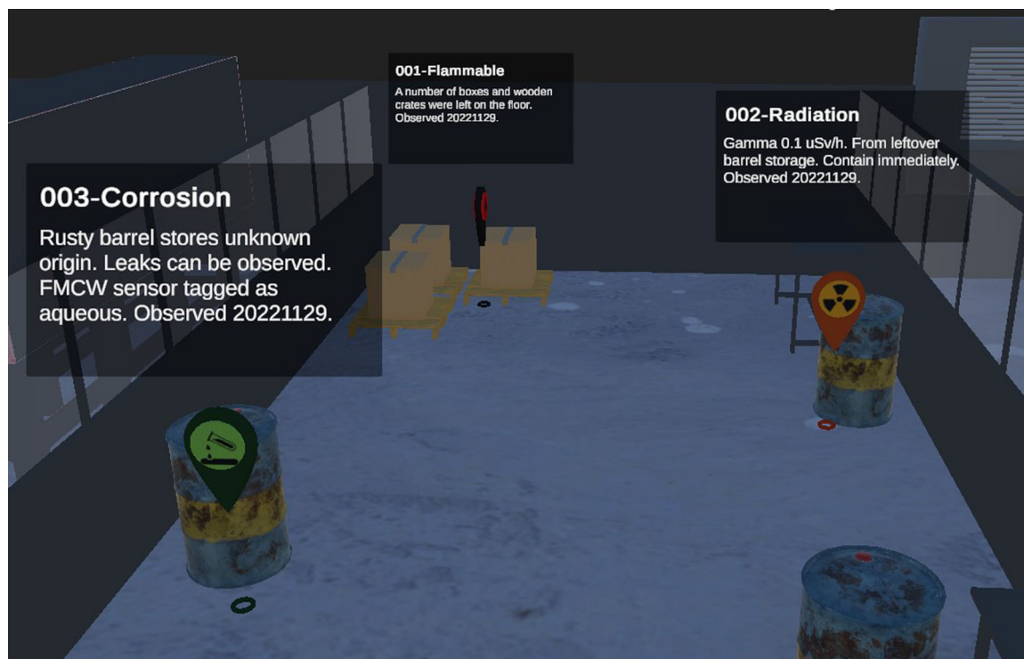
FIGURE 7 Hazard tags and annotations in the digital twin interface. FMCW, frequency-modulated continuous-wave.
