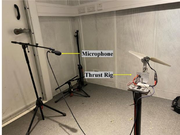
**Fig. 12 Acoustic Testing Setup in UWE Bristol’s Anechoic Chamber**
