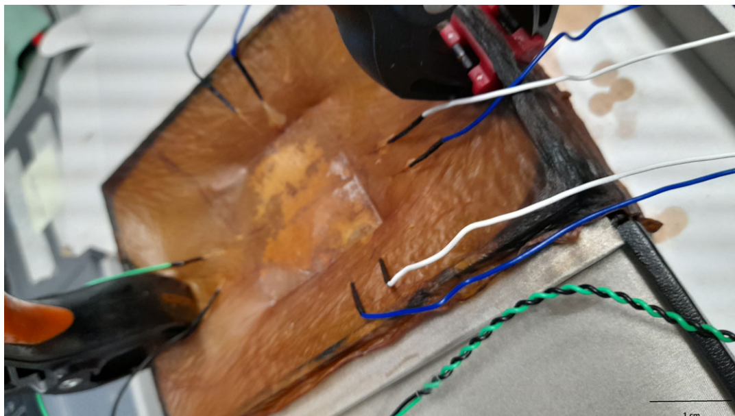
Figure 1. The experimental setup employed for the analysis of electrical spikes in Kombucha using Picolog electrodes. The growth of the Kombucha biofilm proceeds in a sugared tea infusion enriched with the necessary nutrients. Platinum–iridium wire electrodes are inserted into the Kombucha matrix. The electrodes are linked to a Picolog ADC-24 data logger with high impedance capabilities in order to facilitate the capture and storage of electrical signals. The photograph given depicts a magnified perspective wherein the working electrodes are observed to be entering the Kombucha sample. The experimental configuration enables the application of stimulation to the Kombucha culture using the Picolog hardware, while simultaneously measuring the dynamic variations in current and the characteristics of spikes, which serve as indicators of the electrophysiological activity of the biofilm. The scale bar in the image represents a length of 1 cm, providing a reference for the size of the experimental setup and the Kombucha biofilm sample in a wet state.
