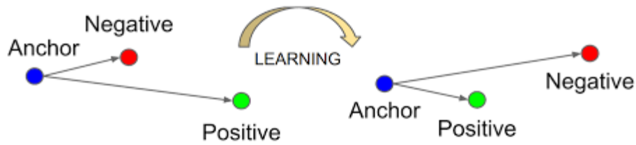
Figure 77: Triplet Loss minimises the distance between anchor and positive and maximises the distance between anchor and negative
