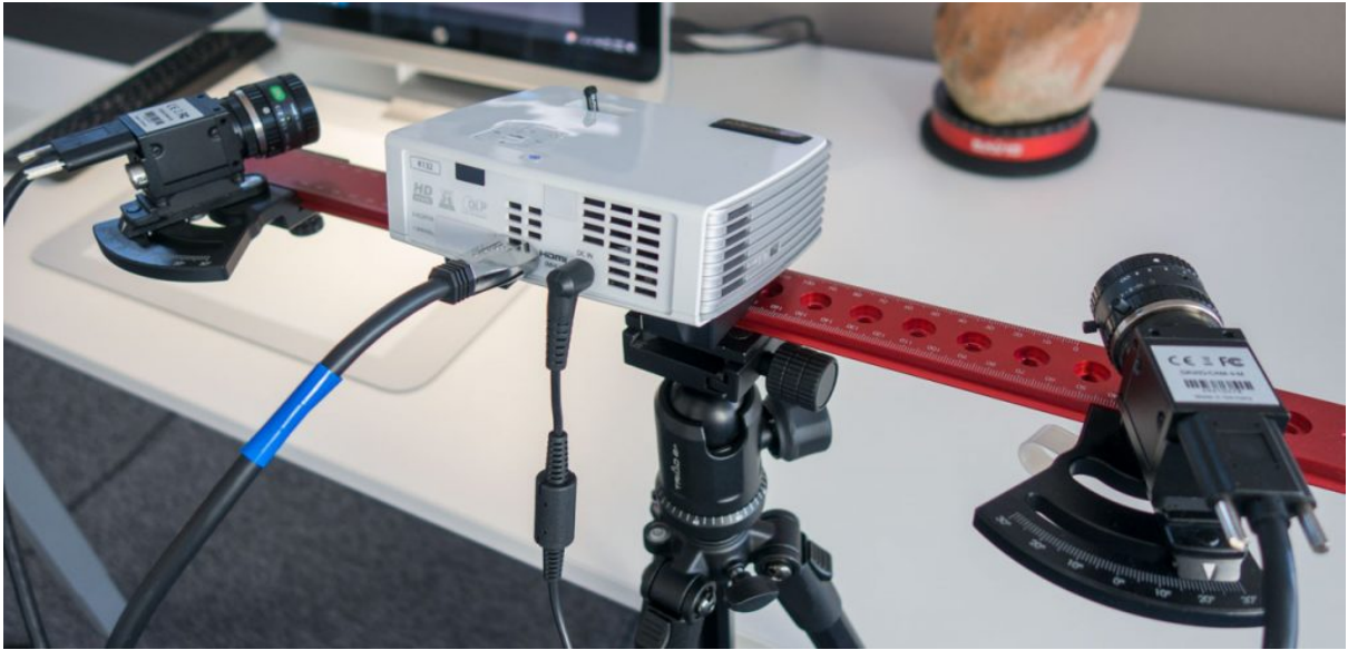
Figure 49: HP Structured Light Scanner Pro S3 (HP, 2023), a structured light scanner that was used for 3D capturing of the 3D printed objects.
