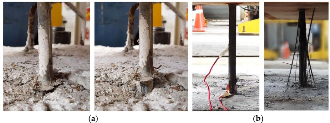
Figure 13. Debonding/Failure of CFRP–Concrete Element: (a) G40 Concrete; (b) UHPFRC.
