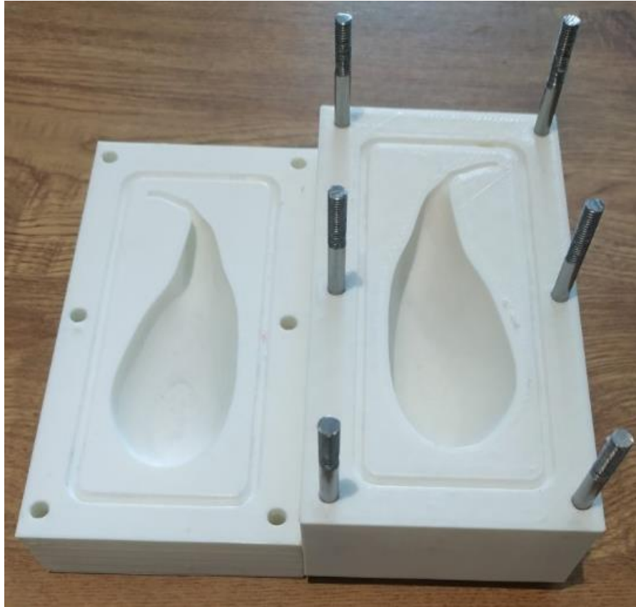
Figure 18: Gallbladder mould and mould clamping system
