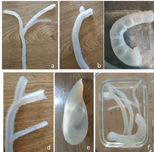
Figure 46: "Fabrication of synthetic soft tissues made of agar gel" by Marine Shao, used under CC BY 4.0
