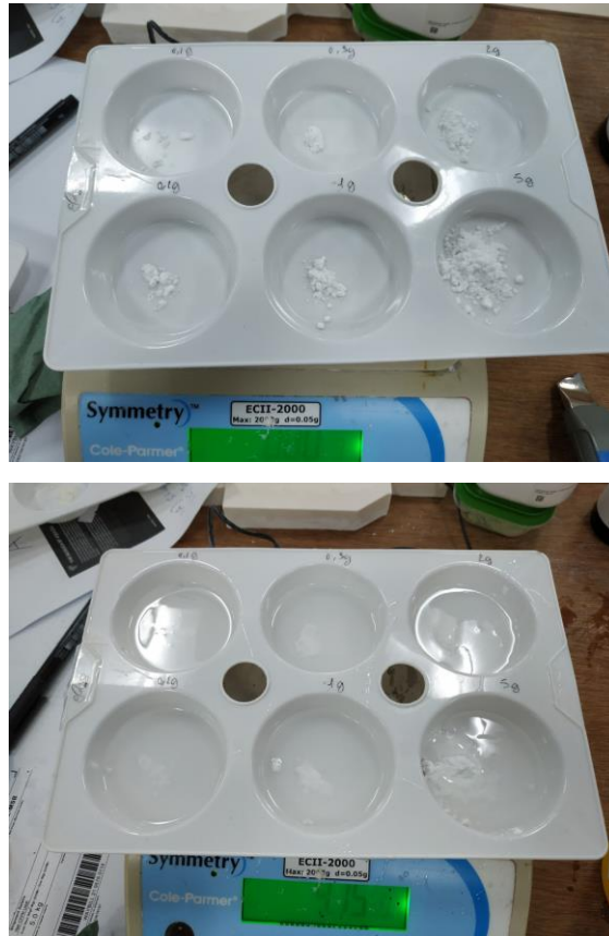
Figure 28: Fabrication of samples using a glass sphere scattering agent and a bulk matrix of DragonSkin
