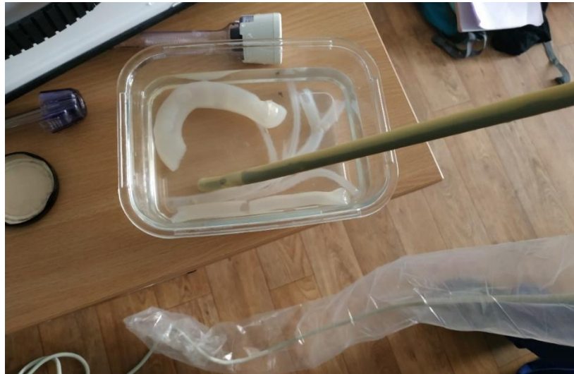
Figure 47: "Recording of the ultrasound images on the agar model using a laparoscopic ultrasound probe" by Marine Shao, used under CC BY 4.0
