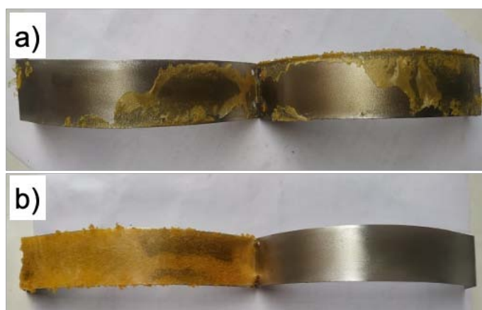
Figure 10: Failure of specimens after T-peel test, a) cohesive failure and (b) adhesive failure
