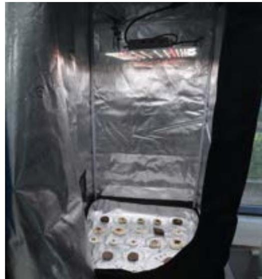
Figure 2: Hydroponic tent used for the lichen-substrate inoculation to allow controlled conditions of light, humidity and temperature for all samples. Photograph by Simon Regan 2023.
