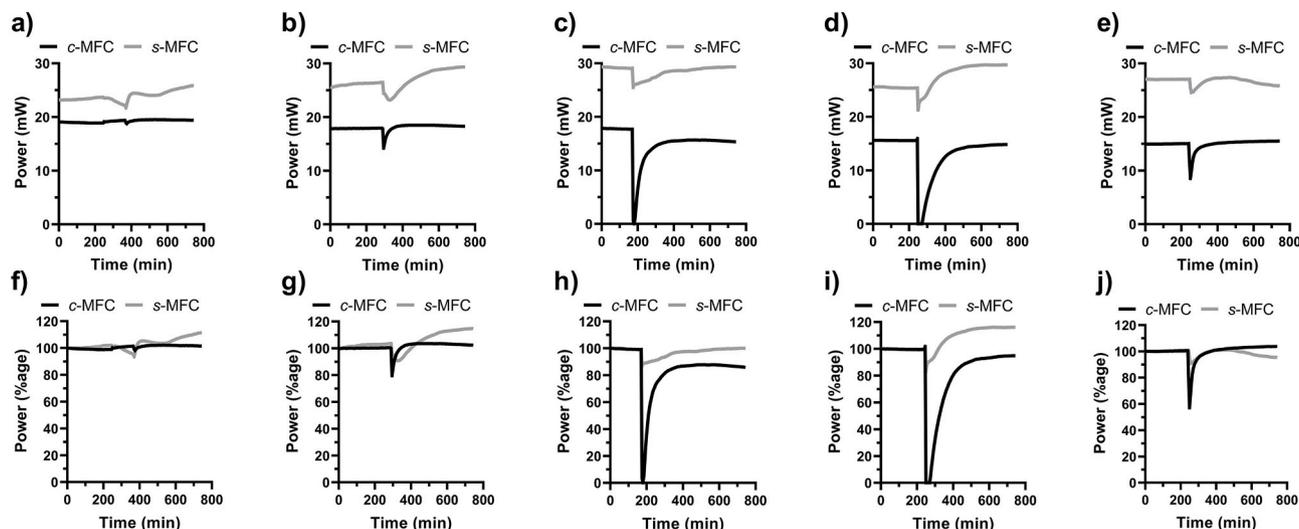
**Fig. 2.** Absolute power outputs under the tested conditions (a,f), and percentage of the output based on the average power produced during the 60 min prior additions. Response of the cascades to the additions of: (a,f) 50 ml of 24 mM NaClO, (b,g) 200 ml of 24 mM NaClO, (c,h) 500 ml of 24 mM NaClO, (d,i) 500 ml of 48 mM NaClO, and (e,j) 50 ml of 605 mM NaClO.
