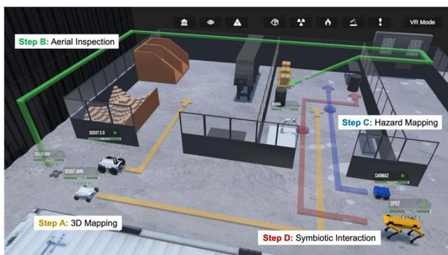
**FIGURE 8** An overview of the semi-autonomous inspection mission as viewed from the DT interface. Robot paths are displayed with coloured arrows matched with coloured text through steps A-B and specific waypoints displayed via circles.
