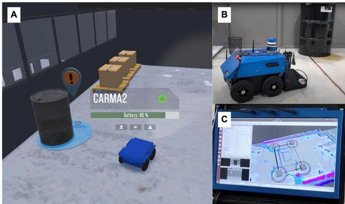
**FIGURE 11** Continuous Autonomous Radiometric Monitoring Assistant (CARMA) UGV provides a map of the hazards in the areas of interest. (a) CARMA localisation within the DT interface, (b) a photo of CARMA in the physical environment, and (c) Data generated by CARMA using its Frequency Modulated Continuous Wave (FMCW), Alpha, and Gamma sensors.
