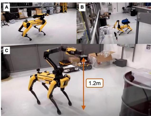
**FIGURE 13** Symbiotic interaction between Spot quadruped and Franks Panda Manipulator (a) Spot moving through environment, (b) Spot collecting the tool from the mobile garage at the Franka manipulator, (c) Spot performing a vertical scan of the surrounding area with the  $\gamma$  sensor.
