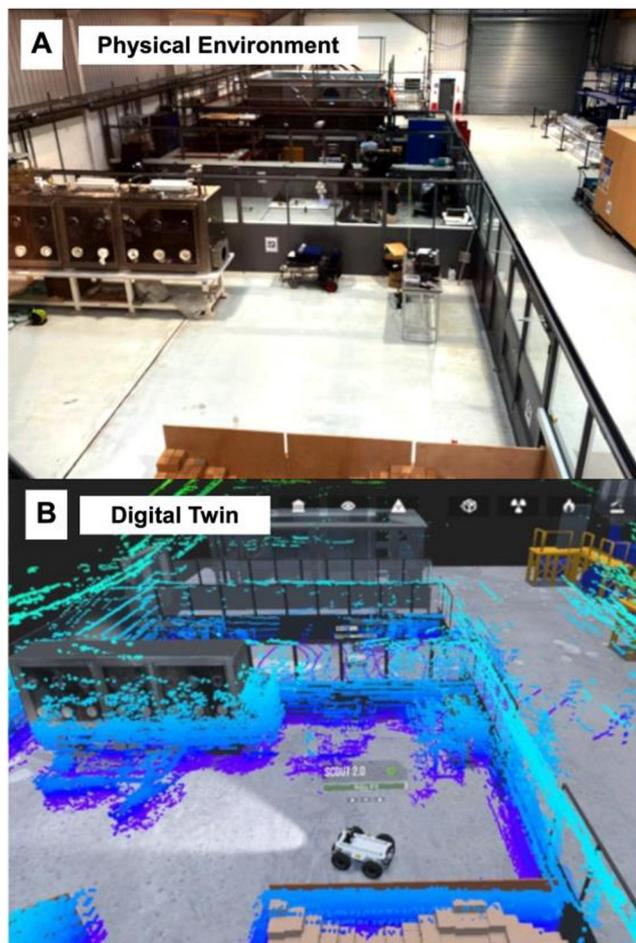
**FIGURE 9** Results of the 3D mapping scenario for the inspection mission of the RAICo1 Facility: (a) the physical environment and (b) the generated voxels overlaid with the existing Building Information Models (BIM) in the DT interface. The 3D mapping data was compared to existing building plans and BIM data to detect dynamic changes to the environment.
