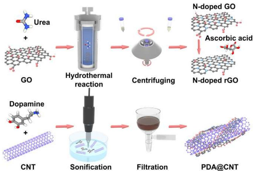
**Figure 10. Schematic diagram of N-doped rGO and PDA@CNT**
