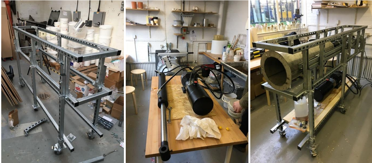
FIGURE 4. The construction of the piston-based extrusion machine used for this study. (Left) The basic frame constructed from Unistrut components. (Centre) The hydraulic power system. (Right) The completed extruder. (Photos: T. Jorgensen, 2019)
