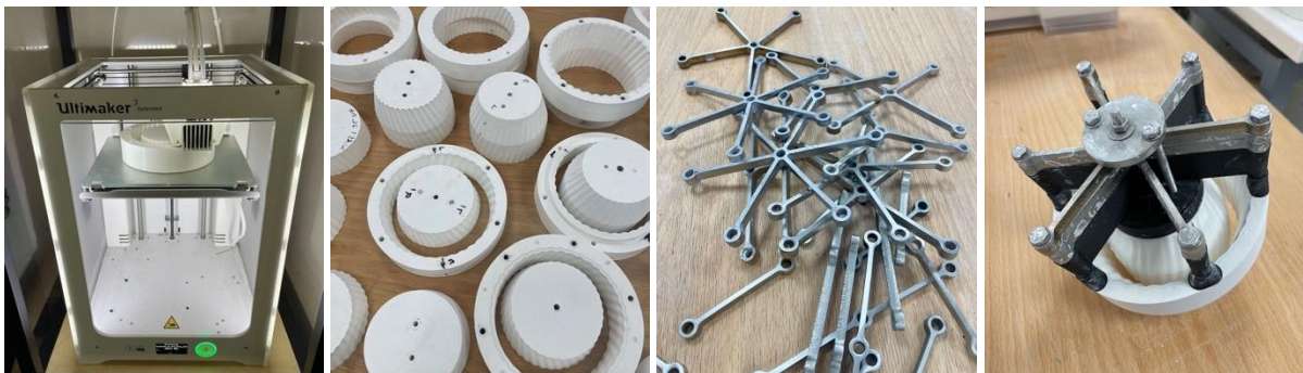
FIGURE 5. The fabrication of extrusion dies using low-cost 3D printers. 3D printed parts were used in combination with bespoke laser-cut stainless steel brackets to enforce the die bridge, the part of the die found to be most prone to failure due to the high extrusion pressures. (Photos: T. Jorgensen, 2022)
