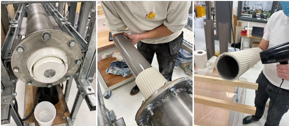
FIGURE 10. Experiments with extrusion using internal support in the form of plastic pipes. In these tests, the extrusion die was fitted with a circular disk to ensure the plastic support pipes would stay in position during the extrusion process. The plastic pipes were heavily lubricated to ensure the clay would slide onto the support without sticking. (Photos: T. Jorgensen, 2022)
