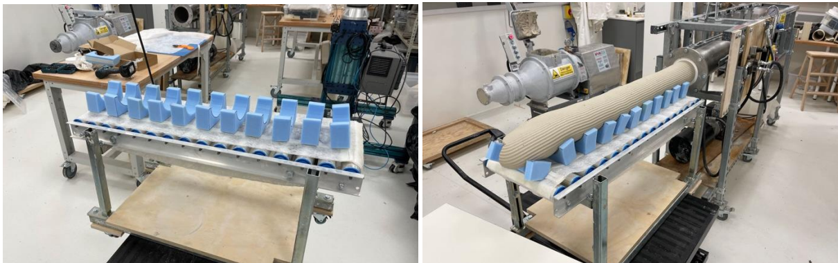
FIGURE 9. Experiments with the use of upholstery foam supports fitted to a manual conveyor belt. (Photos: T. Jorgensen, 2022)
