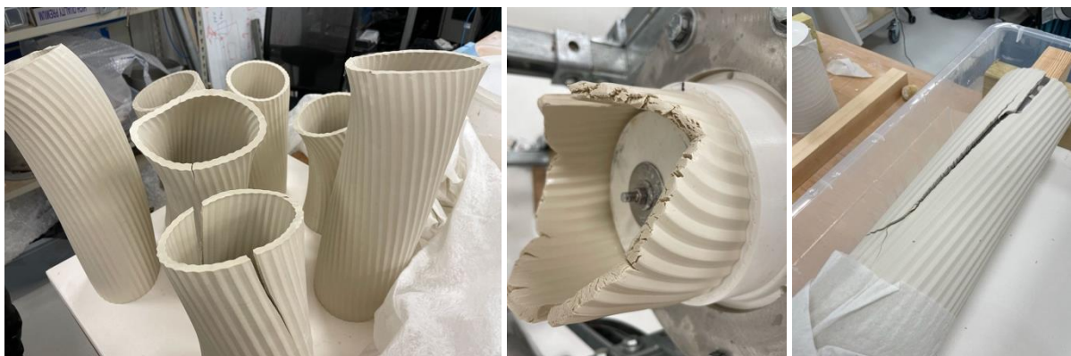
FIGURE 8. Examples of the challenges of extruding porcelain. (Left) Splitting resulting from rapid drying. (Centre) Compression fractures. (Right) Gravity-induced cracks. (Photos: T. Jorgensen, 2022)
