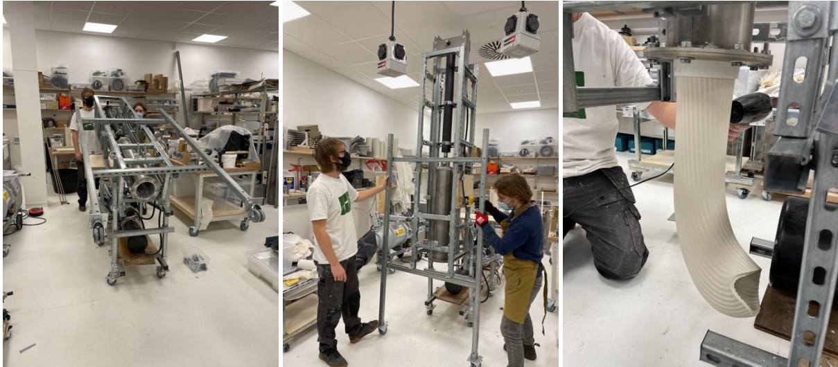
FIGURE 11. (Left and centre) Adaptation of the extruder machine to operate in a vertical position. (Right) A twisting shape being successfully extruded. Initial hardening of the shape was carried out with a hairdryer to enable handling. (Photos: T. Jorgensen, 2022)
