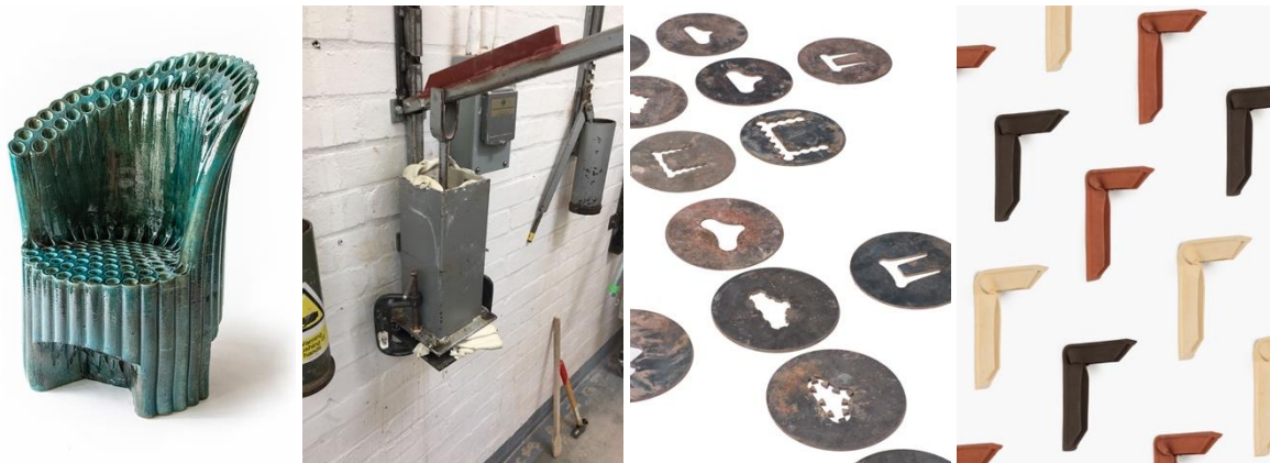
FIGURE 1. Examples of the use of extrusion in craft and design practice. (Far left) Floris Wubben's extruded Throne (2022) (photo: F. Wubben, 2022, permitted reproduction). (Centre left) Small hand-operated extruder commonly used in craft ceramics (photo: T. Jorgensen, 2018). (Centre right) Metal extrusion dies by Studio Apparatu used for Xavier Mañosa's (2018) designs for ceramic shelf brackets (far right). (Photos: Jara Varela 2018, permitted reproduction)
