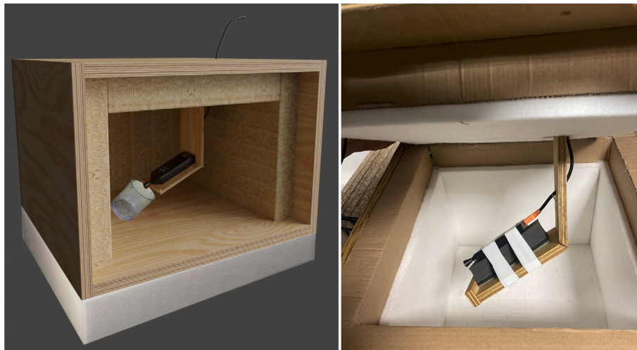
Fig. 2. Left: Render of the high-attenuation acoustic chamber used for recording specimens. The biological specimen is placed within a plastic pot when recording. This rendering shows the front panel removed; in reality, the lid is detachable rather than the front panel. Right: photograph with the lid partly open. The microphone cable is fed through a small hole at the top.
