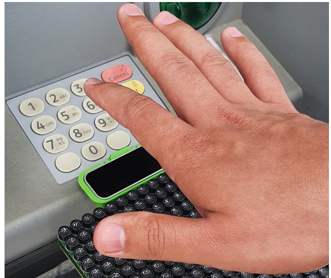
Figure 4: The proposed touchless keypad system for use in situations where private input is needed. The user holds their hand over the keypad in mid-air, where an infrared sensor tracks its movements. A grid of ultrasonic transducers aligned with the user’s palm provides touch feedback in the same relative positions as the keypad buttons.
