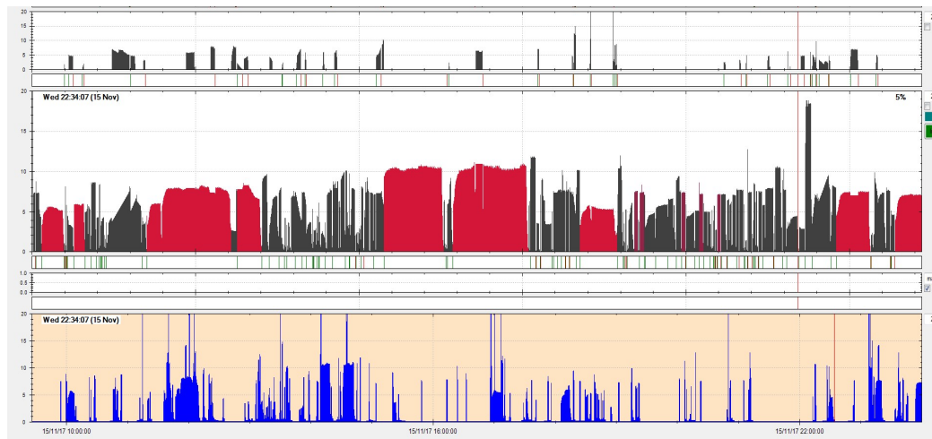
Figure 3-12 Screen shot of Siloette user-interface interface for 20-day test flow trace with shower components (in red) (Source: Rogerson and Spey, 2018)
