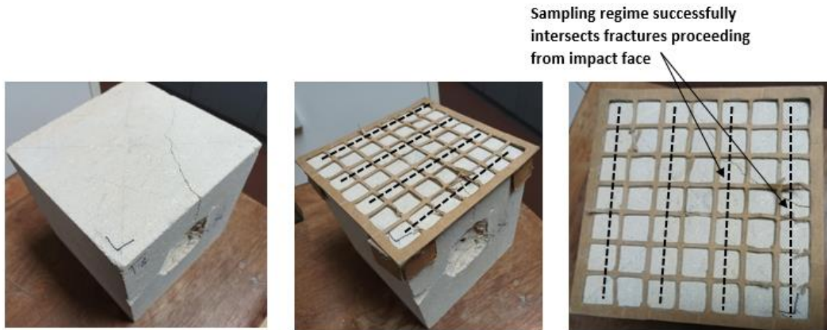
Figure 5.12: The permeability sampling regime on non-impact sides, showing the 28 cells sampled and how they successfully intercept and detect fractures initiated on the impact face from the impact crater.
