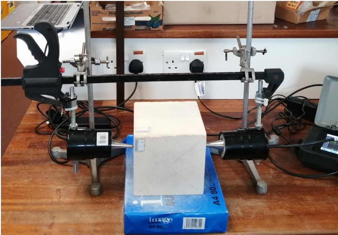
Figure 4.8: The rig used to ensure consistent positioning of the transducers during UPV measurements.
