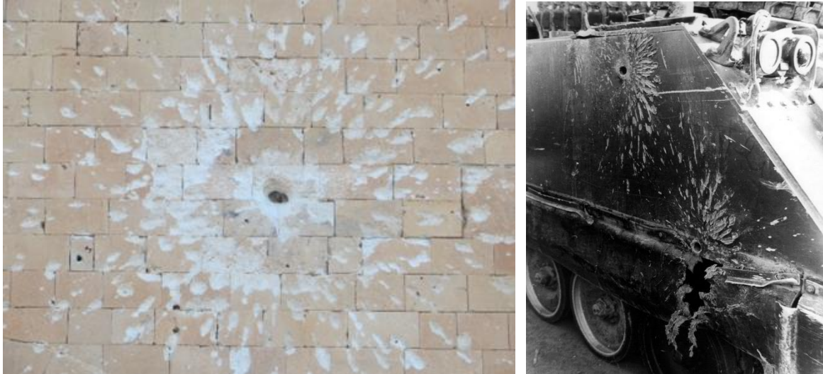
Figure 7.10: A comparison between the RPG impact on the East wall of the amphitheatre (A) (B) and HEAT warhead impact into an armoured vehicle from the Vietnam war. Adapted from Bryla and Starry, 1979.
