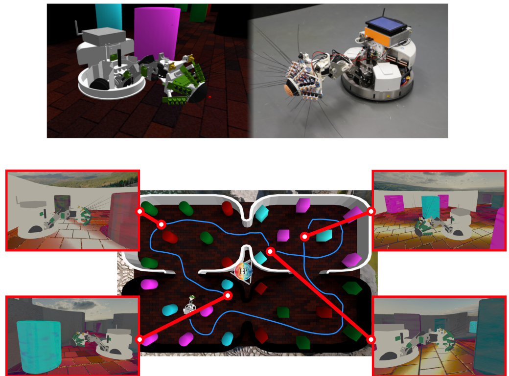
Figure 1. WhiskEye is a biomimetic robot platform that mimics the sensory systems and behaviour of rats and shrews. It has been recreated in simulation along with rich visuo-tactile environments. Exploring these environments autonomously, it gathers multisensory datasets along with odometry data describing its trajectory. These ‘experiences’ of the environment are later used as corrective inputs.
