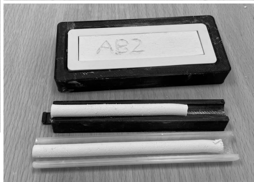
Extrudability and shrinkage tests
