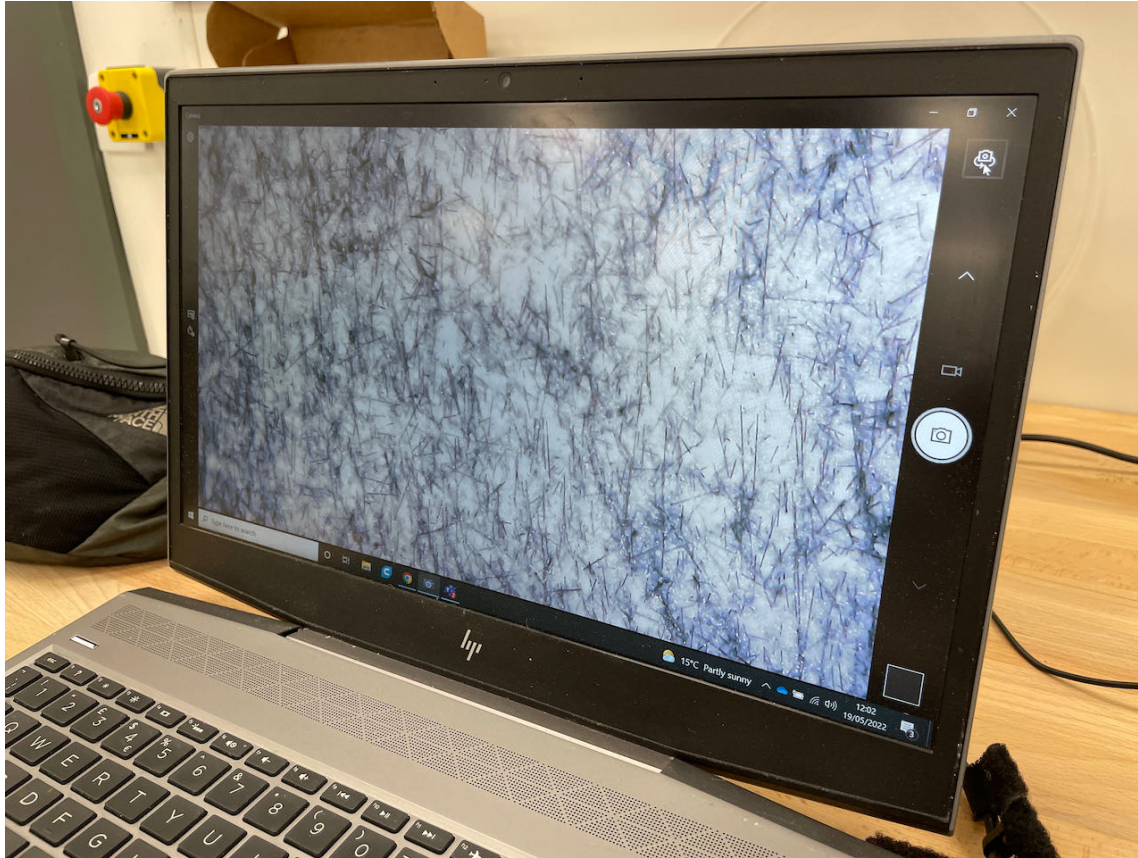
200 X magnification (10 % 6mm Carbon fibre)
