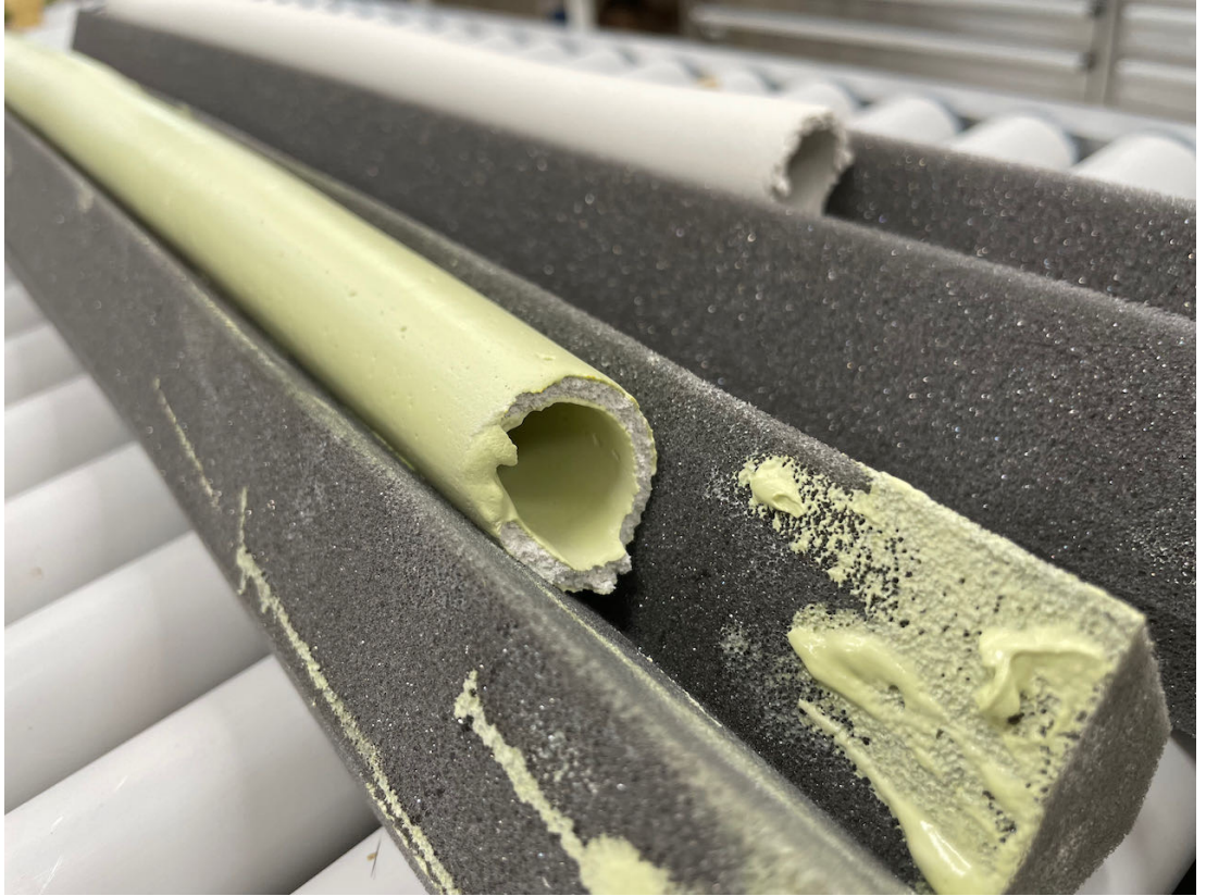
Integrated coating of extruded CNC (internal and external)
