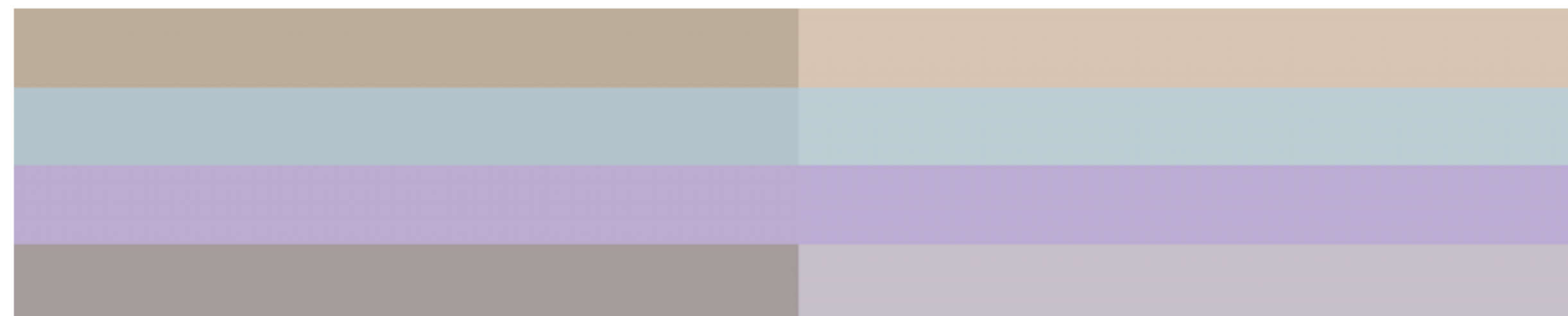
Figure 5. Measured (left) and calculated (right) RGB values of halftoned patches of combinations of primaries under 30° illumination and observation angle. Top to bottom: RG, GB, RB and RGB.
