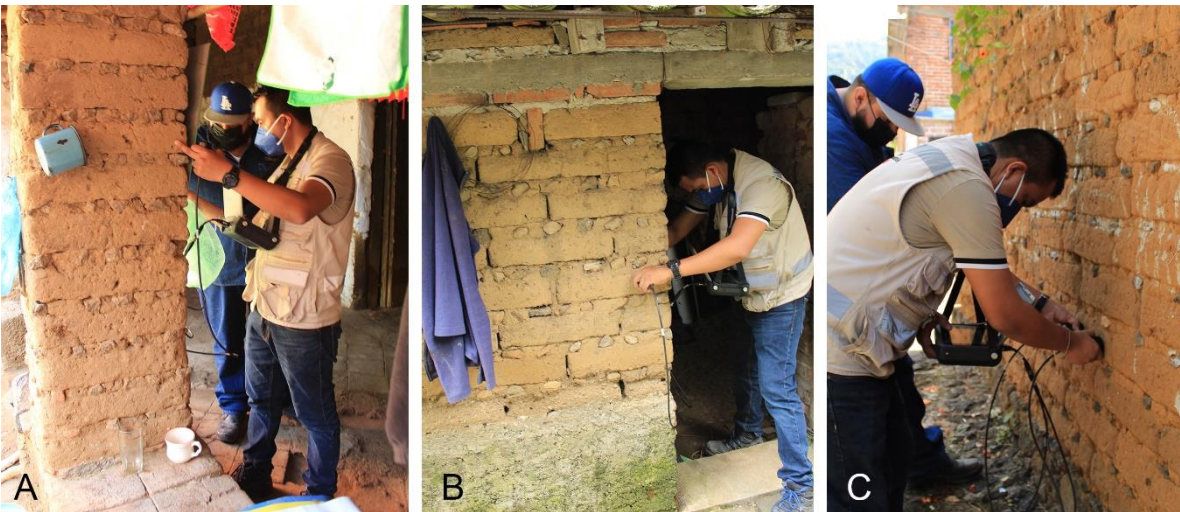
Figure 1. Examples of direct ultrasonic wave propagation measurements in a column (A) and a wall (B) and an indirect measurement in the external face of a façade wall (C)
