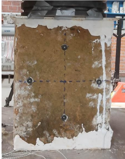
Figure 5. Schematisation of the infrared LEDs array.
