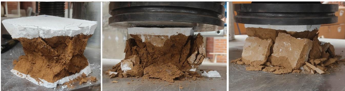
Figure 9. Examples of the failure mode of samples A, B and C, with the detachment of the external layers of material.
