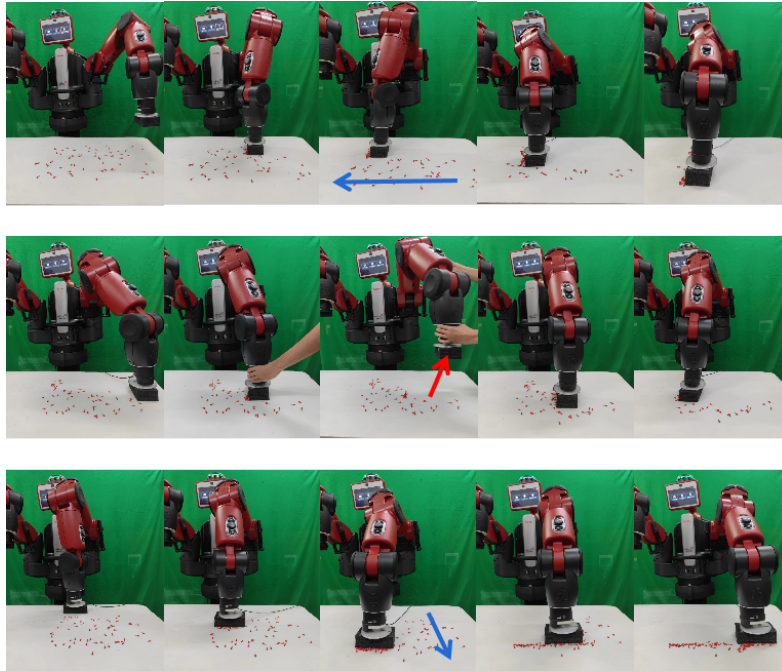
Fig. 6. The first and third lines show the robot completing tasks from different directions, the blue arrow shows the sweeping direction, and the second line shows the robot returning to the sweeping position after encountering the disturbance and continuing to perform tasks.
