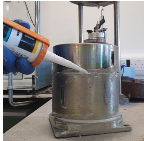
Sealing joints of CBR mould with sample using silicon gel ready for swell test
