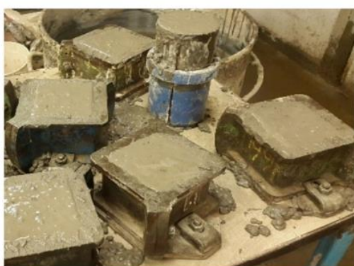
Fig. 3 Fresh concrete in a steel mould
