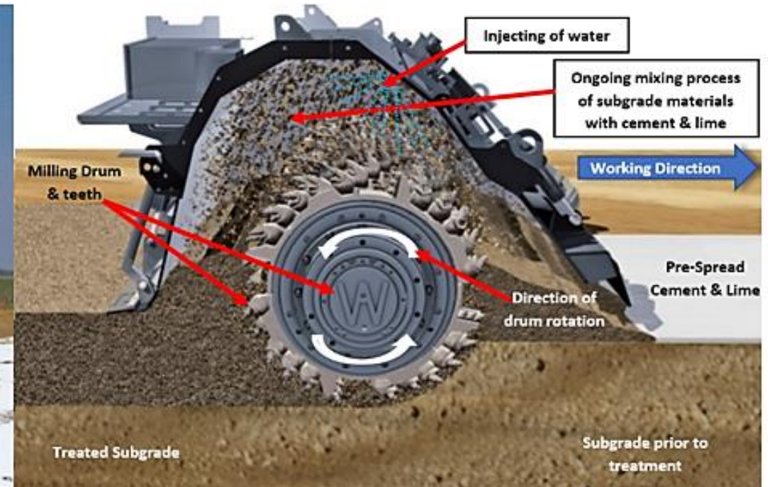
Insitu soil treatment process in mixing chamber (Wirtgen-group.com, 2021)
