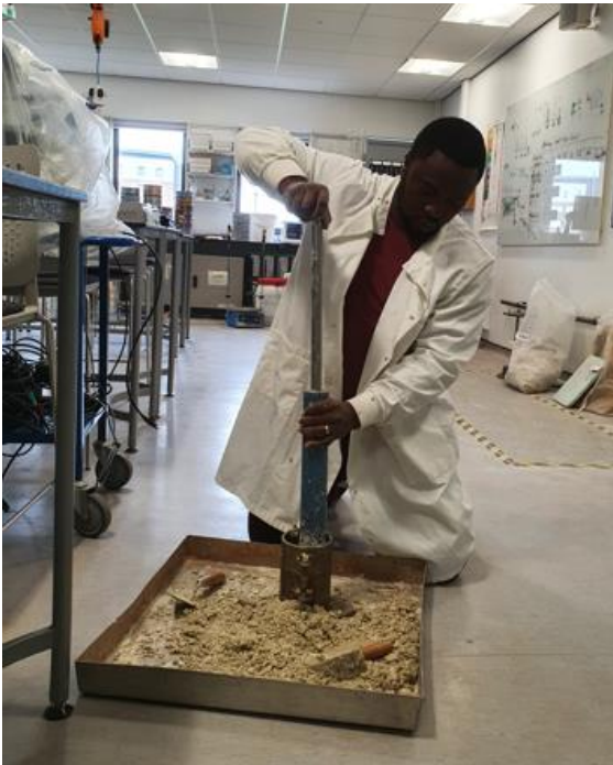
Proctor compaction test sample preparation
