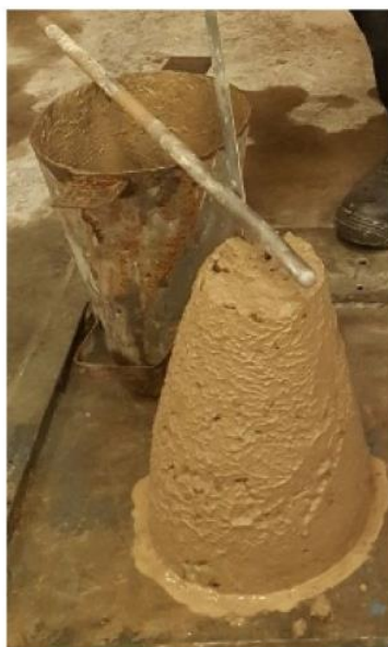
Fig. 6 Laboratory slump test
