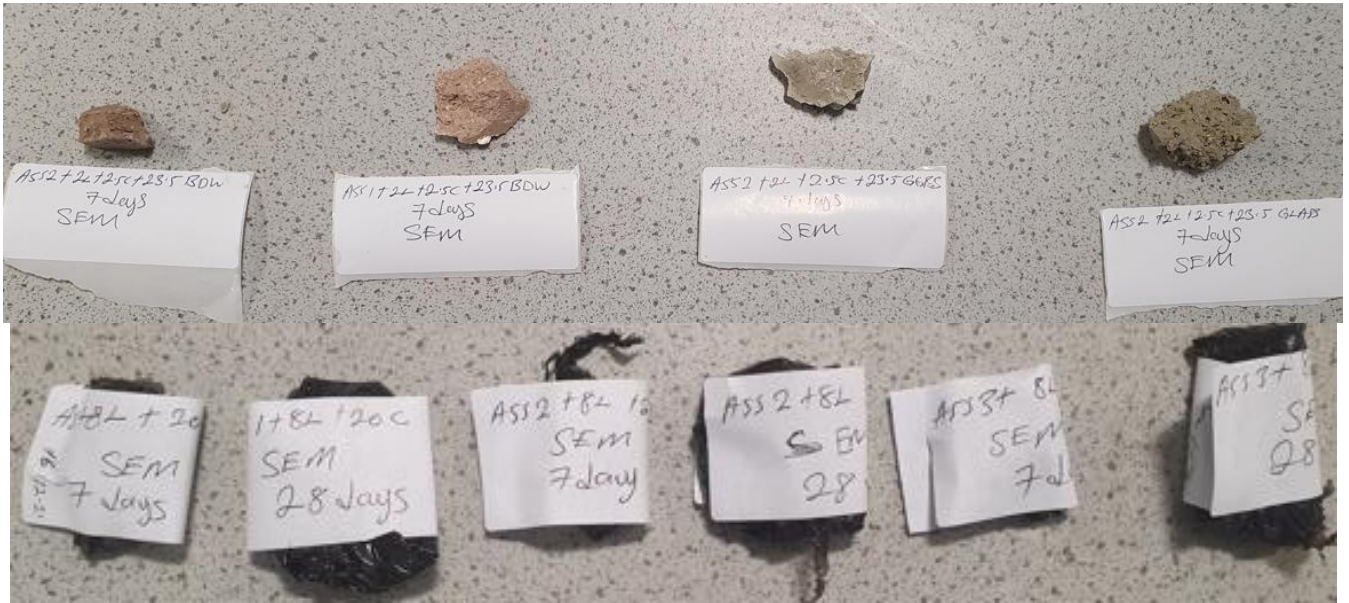
SEM and EDX samples prepared and ready for testing
