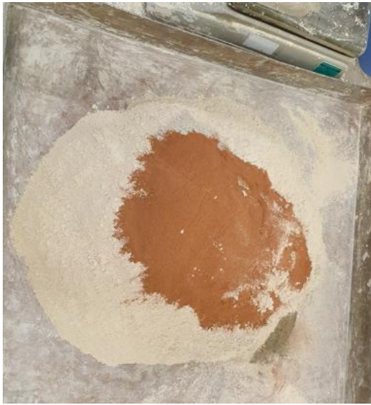
Brick dust waste and other binders added to subgrade material during the mixing process
