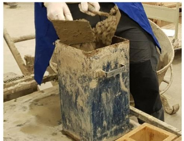
Fig. 7 Filling mould with fresh concrete
