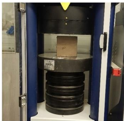
Fig. 10 Applying vertical force to cube specimen
