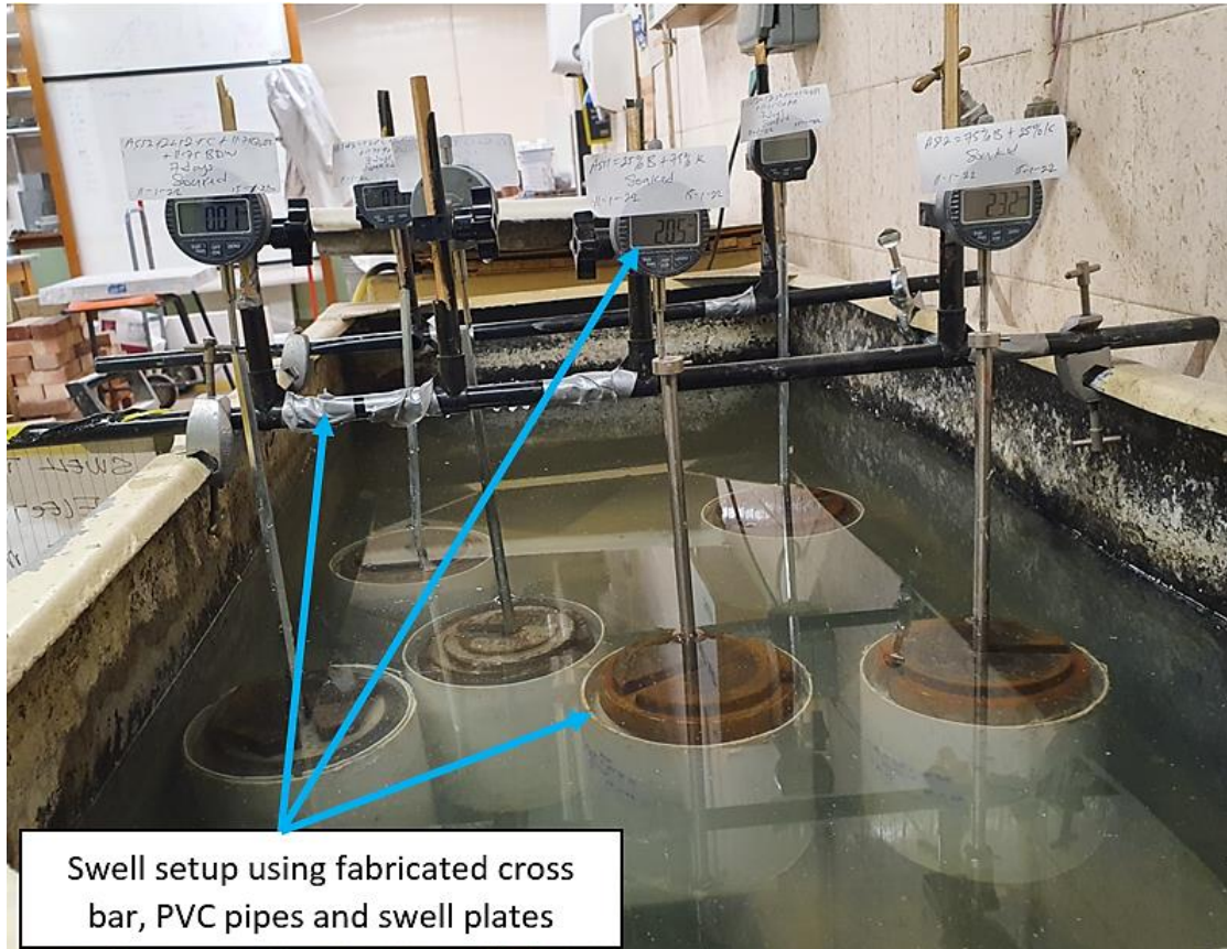
Swell setup using the fabricated crossbar, PVC pipes and swell plates
