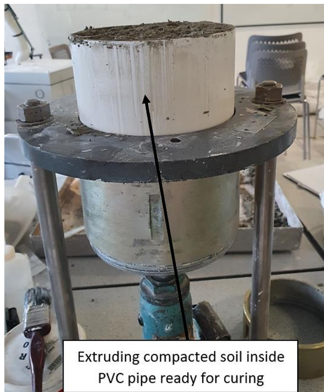
Extruding compacted soil inside PVC pipe ready for curing
