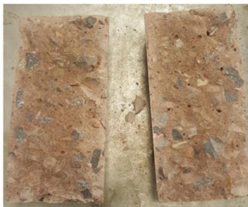
Fig. 14 Failed cylindrical specimen
