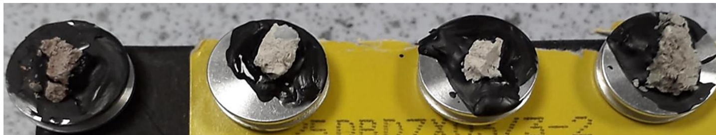
Figure 4.19: Treated Artificially Synthesised Subgrade (ASS) material mounted and ready for SEM and EDX analysis.
