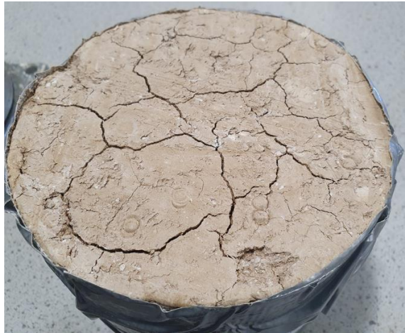
Figure 5.50: Oven dry sample exhibiting cracks similar to a typical existing naturally dry expansive
