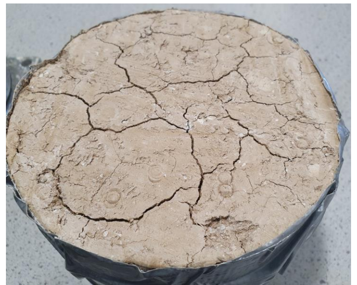
CBR sample cracking due to cyclic drying
