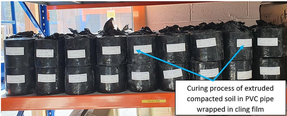
Curing process of extruded compacted soil in PVC pipe wrapped in cling film
