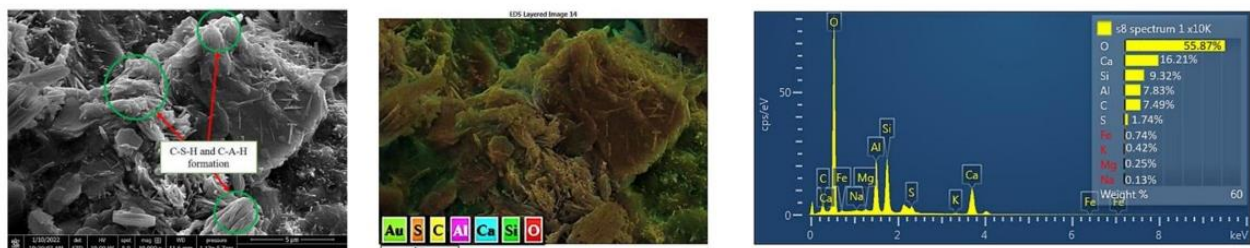
Fig. 2. SEM image, Map and EDX results for ASS1 after 7 days of curing.
