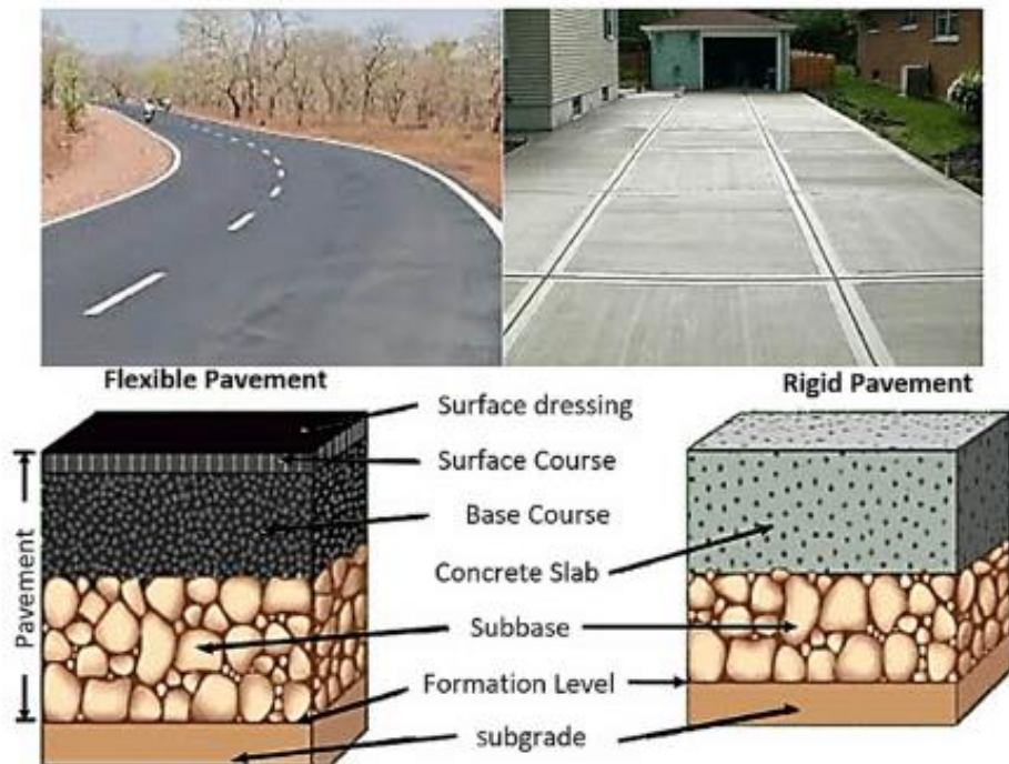
Figure 5. Difference between flexible and rigid pavement [33].
