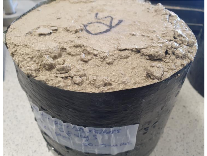
CBR sample eroded after due to cyclic wetting
