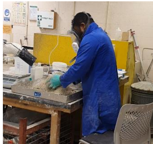
The mixing process of treated subgrade materials
