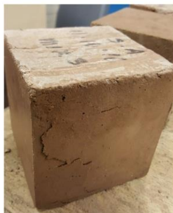
Fig. 11 Failed cube specimen with cracks
