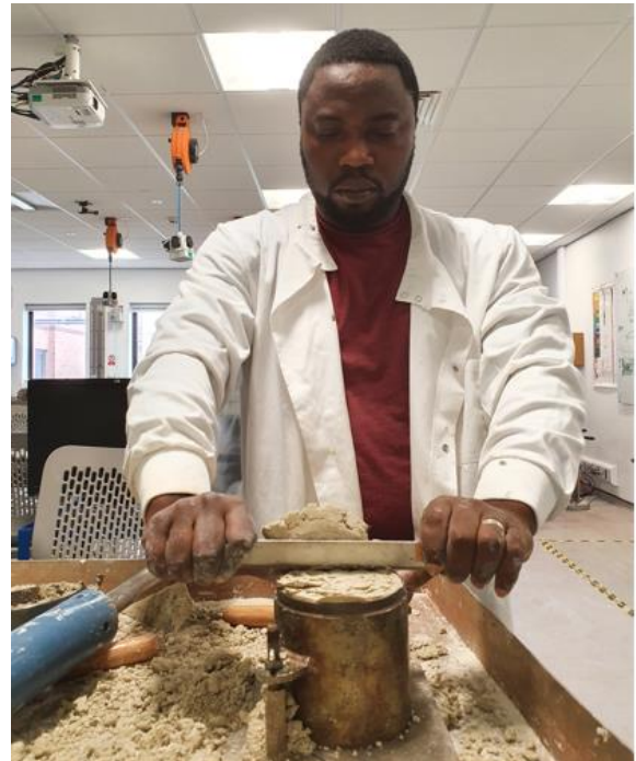
Proctor compaction test sample preparation
