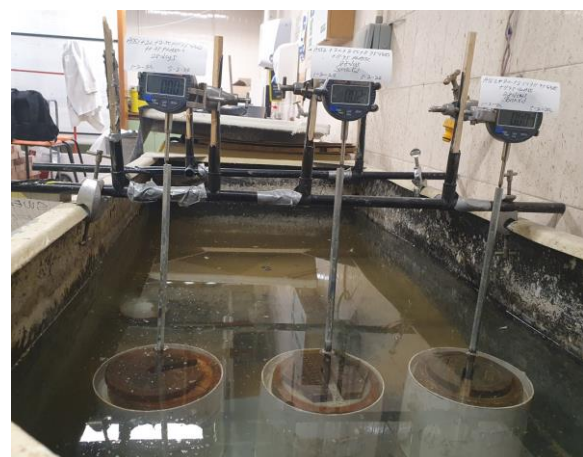
Sealing joints of CBR mould with sample using silicon gel ready for swell test
