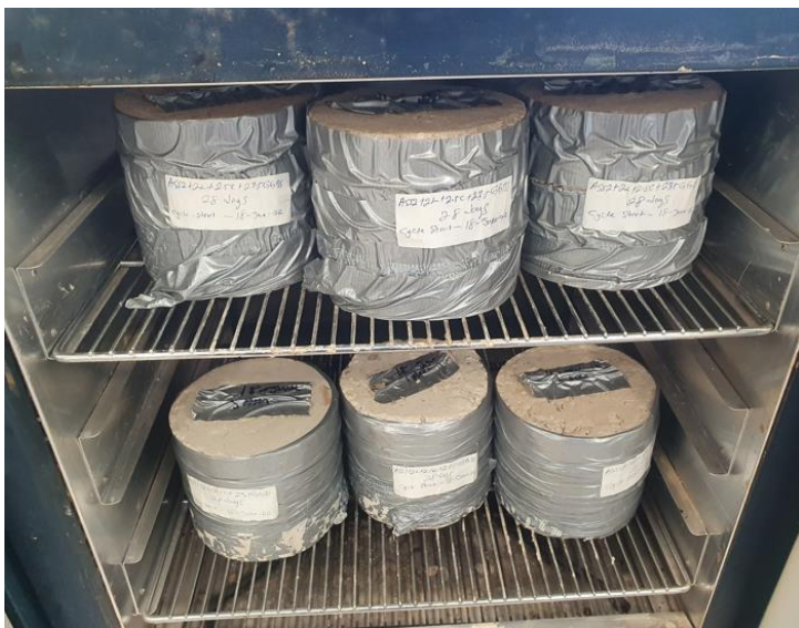
Oven-drying samples for drying cycle test
