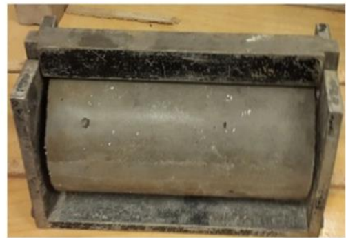
Fig. 12 Cylindrical specimen locked in steel frame
