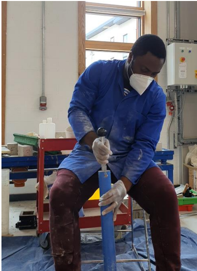
Manual CBR test sample compaction Process
