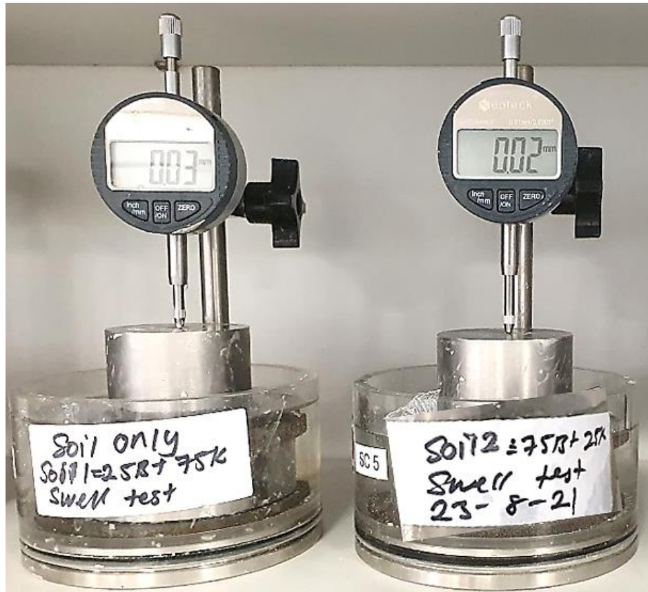
Figure 4.14: Swell set-up for treated and untreated ASS materials
