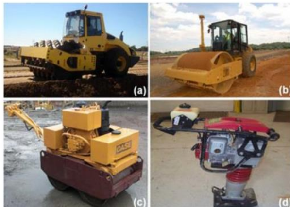
Fig. 8. Different types of compactions (a) Pad-foot or tamping-foot roller (b) Smooth-drum vibratory roller (c) Walk-behind vibratory compactor and (d) Jumping-jack tamper (Meehan et al., 2009).
