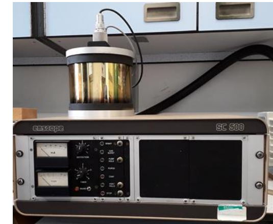
Figure 4.18: Gold Sputter Coating Unit.
