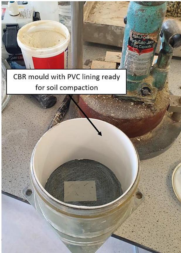
CBR mould with PVC lining ready for soil compaction
