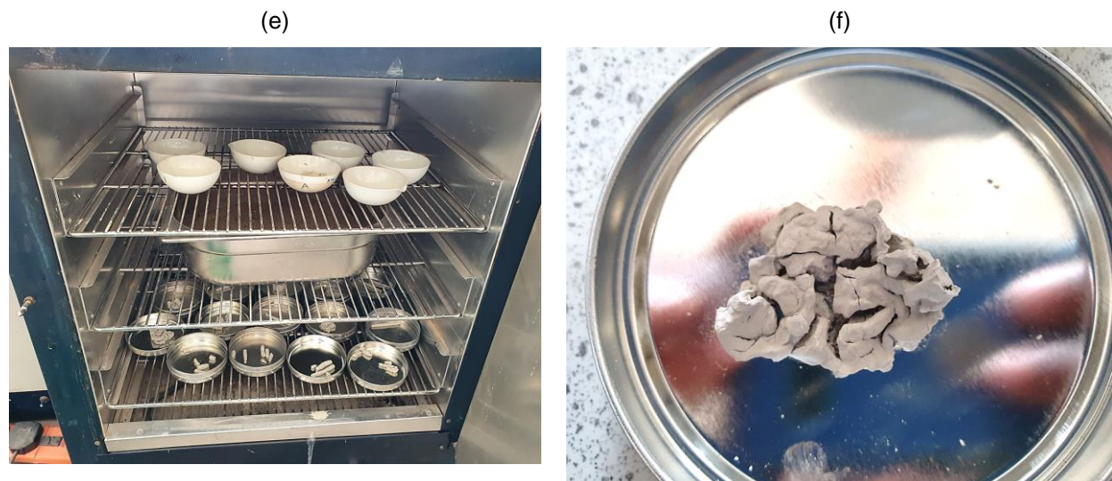
Figure 4.3: Laboratory test process and how liquid limit samples were prepared (a) Testing pH level of water used (b) Soil at liquid limit state (c) Cone penetration process during liquid limit test (d) Taking specimen after cone penetration for liquid limit test (e) Specimen and container on a scale (f) Wet specimen in containers ready for oven-drying (g) Specimen in the oven (h) Oven-dried specimen in containers
