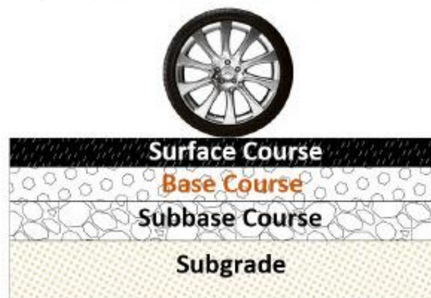
Figure 6. Three-layer flexible composite pavement structure.
