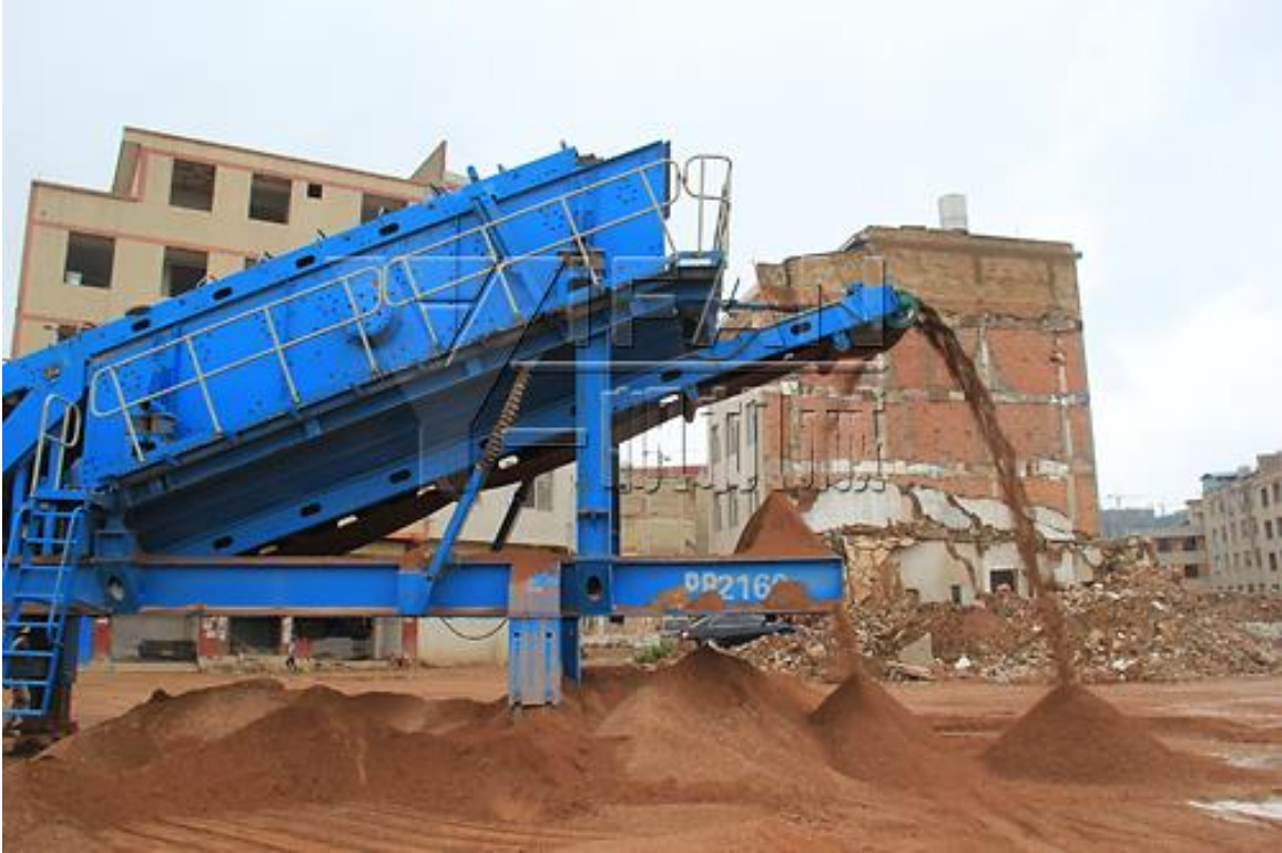
Figure 2.20: Recycling of brick waste to produce brick dust waste (YiFan concrete crusher, 2012)
