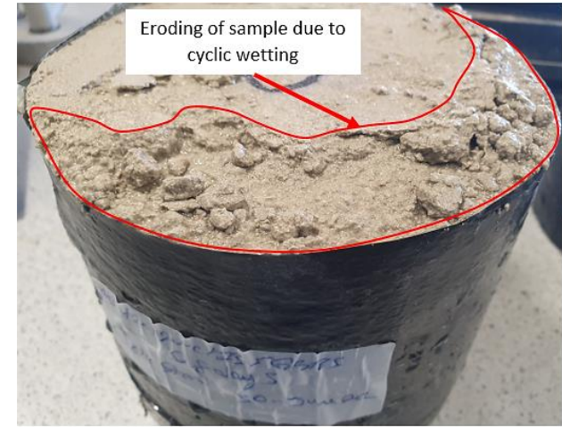
Figure 5.52: Eroding of sample due to cyclic wetting
